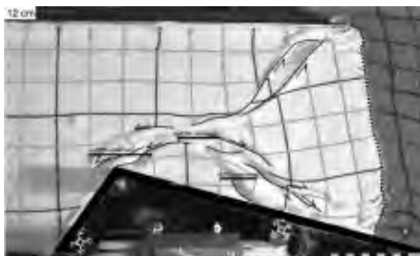
Fig. 4: Surface of 3-layer model with thickened ductile crust. Oblique convergence ( 20^\circ to the NNE).
