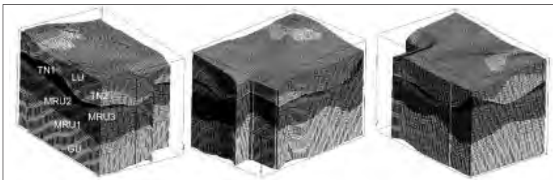
Fig. 3 - Different views of the obtained structured grids for the study area. Note the boudinage affecting the TN and UMR3 tectonic units.
