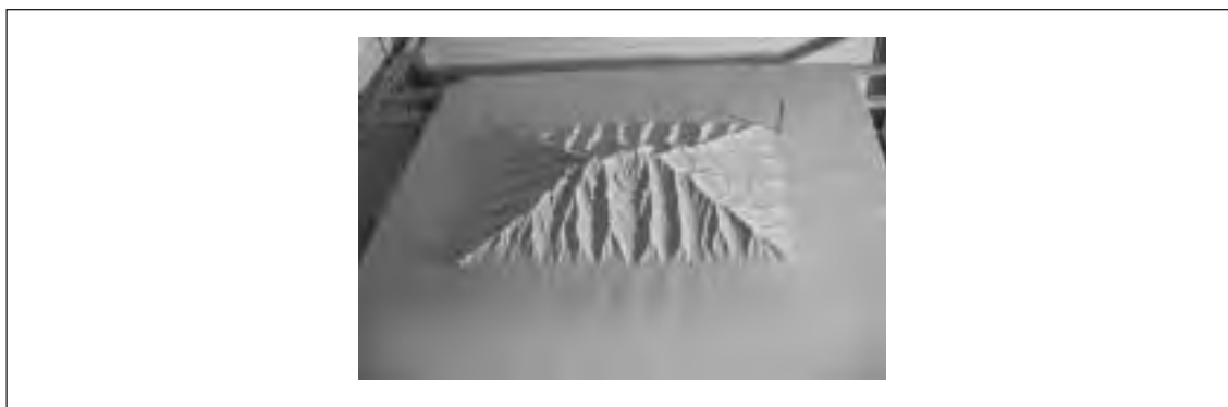
Figure 4 - Photograph of experiment of erosion of an uplifted relief associated with the foothill deposition of the eroded products.
