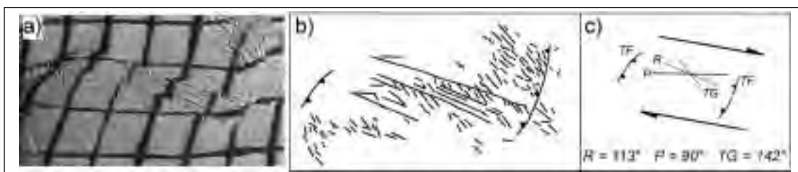
Fig. 4 - Fault-related fractures developed in model DR02 (a), between domains B and C. Black squared grid is 2 cm. (b) Line drawing of interpreted fractures. (c) Sketch of the interpreted Riedel system, showing a dextral shear with an azimuth of 100°. TF: thrust fault; R: synthetic shear; P: low angle synthetic shear; TG: tension gashes.
