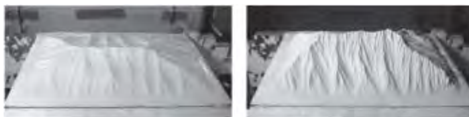
Figure 3 - Examples of small-scale (14 x 20 cm) experiments at steady-state with the same uplift rate (15 mm/h) but under high (left: 165 mm/h) and low (right: 100 mm/h) rainfall rates.
