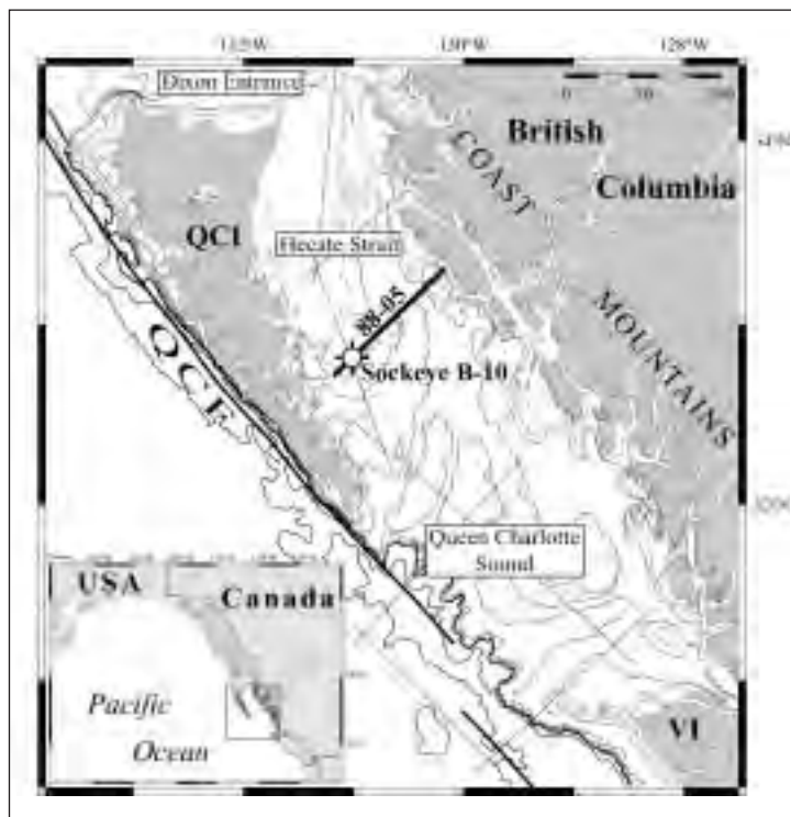
Fig.1 - Location map of the area under study. Approximately 1000 km of reflection seismic lines have been recorded by the Geological Survey of Canada (Rohr and Dietrich, 1992)). This study focuses on line 88-05 (bold) and offshore well Sockeye B-10 (Shell Canada). Queen Charlotte Fault (QCF), Queen Charlotte Islands (QCI), and Vancouver Island (VI) are marked.
