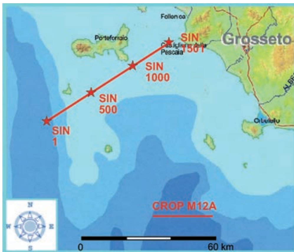
Fig. 1 - Location map of the M12A CROP profile. The location of four shots along the line are highlighted by red stars. The water depth is approximately 90 m for the most part of the line while it deepens to 800 m in the western part of the line (Corsica basin).
