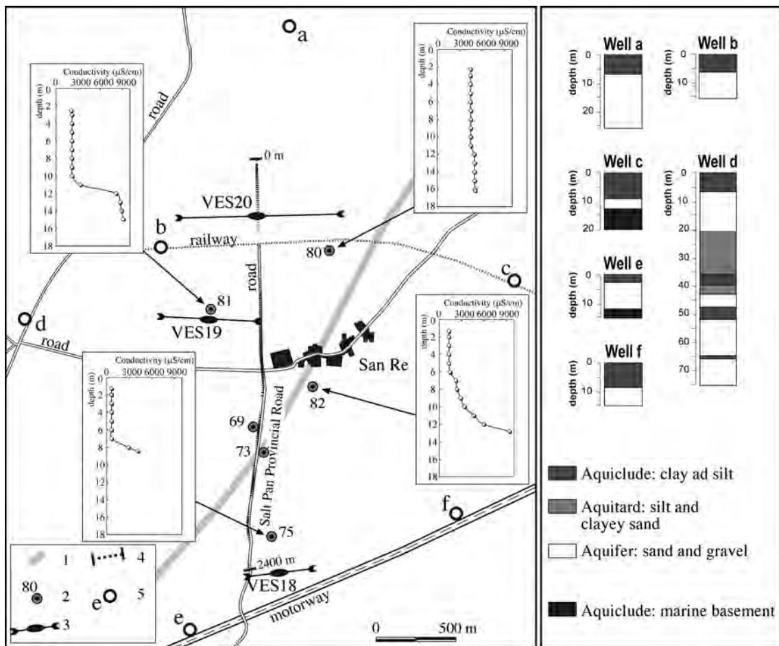
Fig. 13 - Investigation undertaken within the selected site shown in Fig. 3 legend: 1) trace of the Vogherese Fault (assumed from pre-existing investigations) in plan view; 2) well; 3) VES; 4) resistivity profile and VLF line 29; 5) well with stratigraphy.
