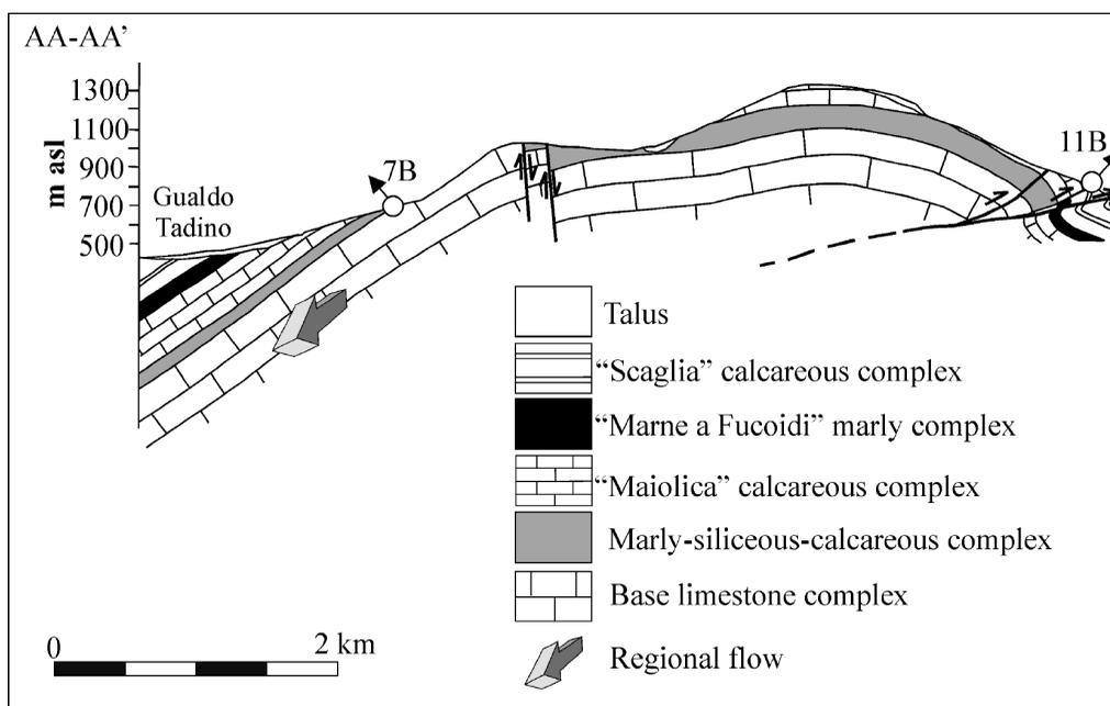
Fig. 4 - Hydrogeological cross-section through Gualdo Tadino anticline.
