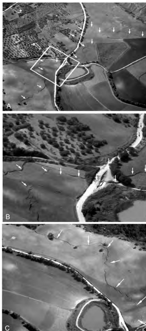
Fig. 2 - Aerial panoramic views of the Cerda landslide main scarp some days after the September 6, 2002 reactivation (by INGV): a) “M-shape” main scarp (the white square shows the area zoomed in Fig. 2b); b) secondary scarps and damage along a side road; c) detail of the main scarp (southeastern side).
