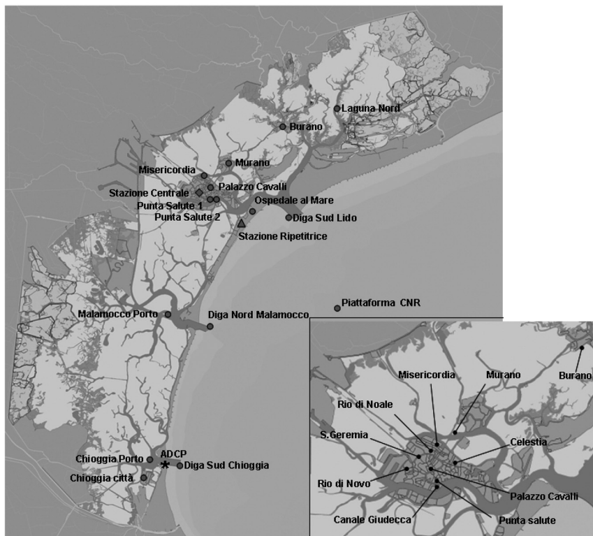
Fig. 2 - The ICPSM's monitoring network. In the little box on the right the wave gauge network is visible. The current meter at the Chioggia inlet is marked by a star.
