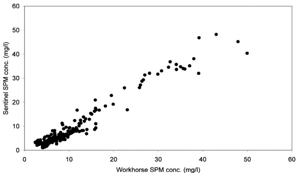
Fig. 14 - Calibration of the bottom-mounted ADCP (y-axis) with indirect concentration estimates provided by the boat-mounted ADCP (x-axis).
