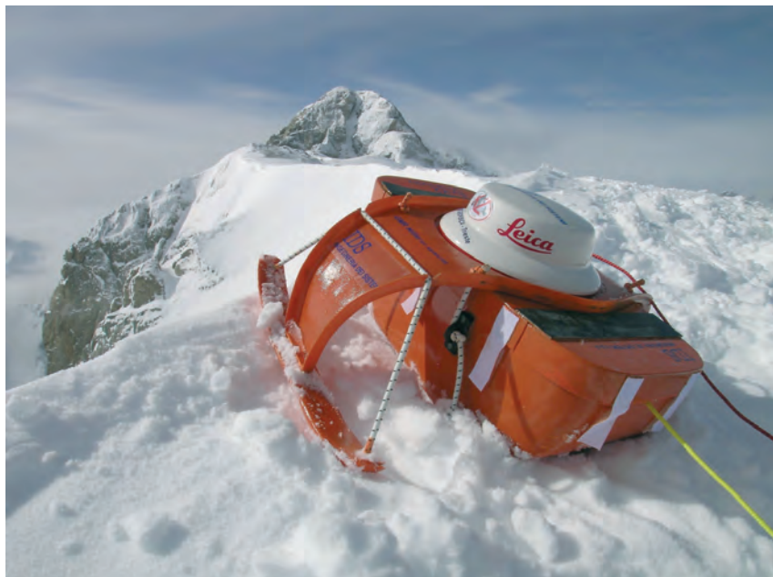
Fig. 3 - April 2004: the first prototype of an IDS georadar coupled with a Leica GPS.
