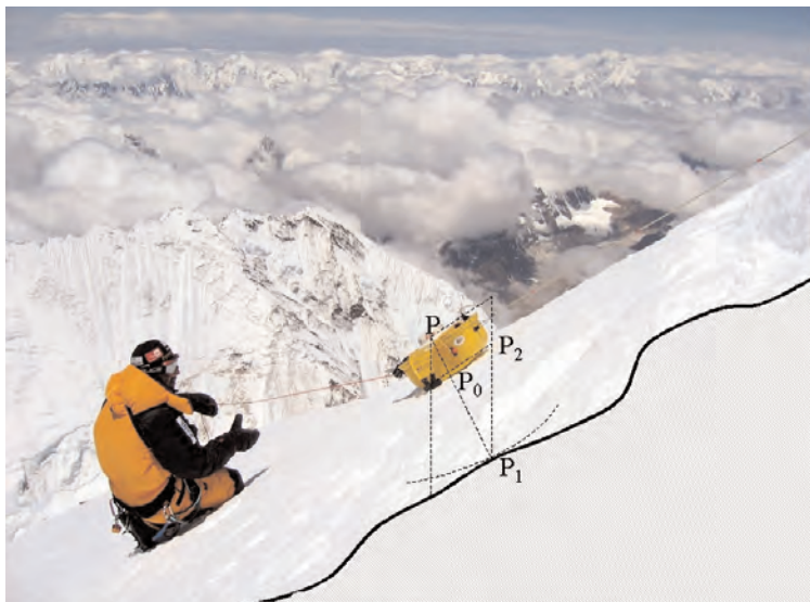
Fig. 10 - Climber Mario Merelli operating the GPR on the steep slope along the SW ridge (foto K. Unterchircher).
