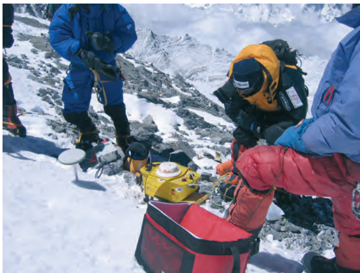
Fig. 8 - The start of the master GPS (static) station and of the GPR/GPS (mobile) in correspondence to the rock outcrop on the southern slope under the summit of Mt. Everest (photo K. Unterkircher).
