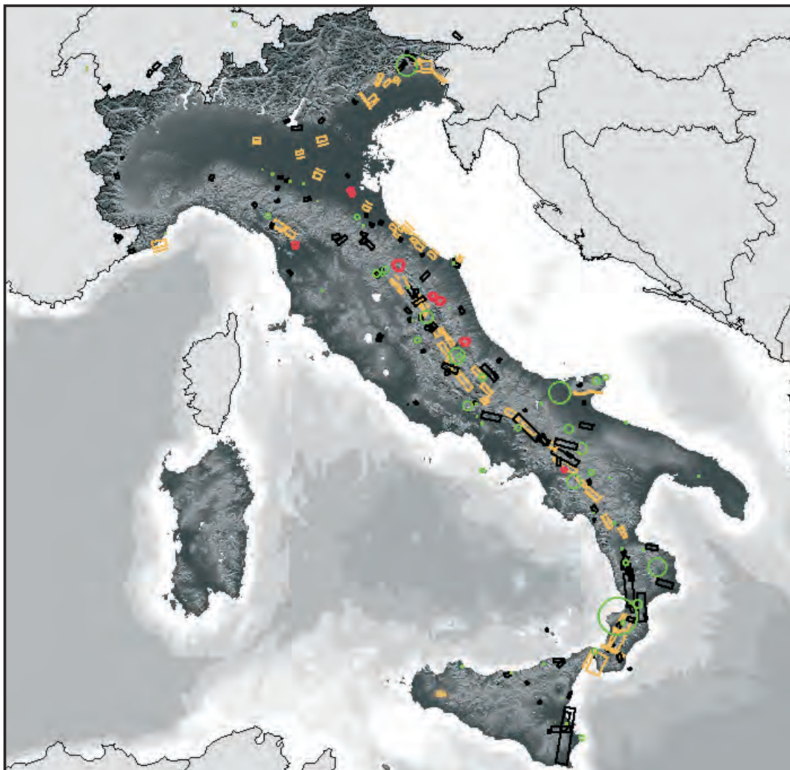
Fig. 1 - Database of Italy's Seismogenic Sources (DISS), version 2.0.516 released at the beginning of the GNDT project (Valensise and Pantosti, 2001): the integrated dataset addresses four kinds of sources: the geological ones (yellow rectangles), the historical well-constrained sources (black rectangles), the historical badly-constrained sources (green circles), the deep sources (red octagons).
