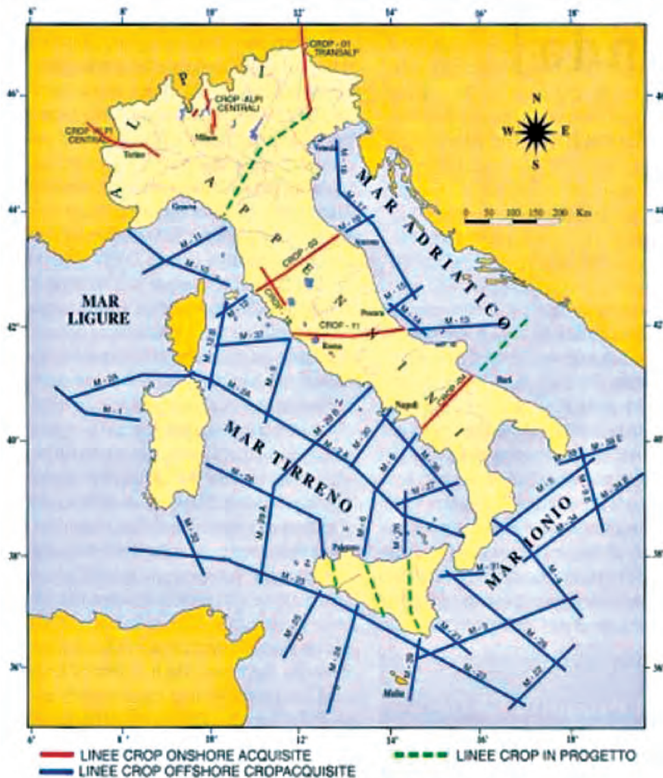
Fig. 6 – The Near Vertical Seismic Reflection CNR Project “CROsta Profonda” in Italy (land: 1450 km, 1996-2004; sea = 8700 km, 1991-1996).
