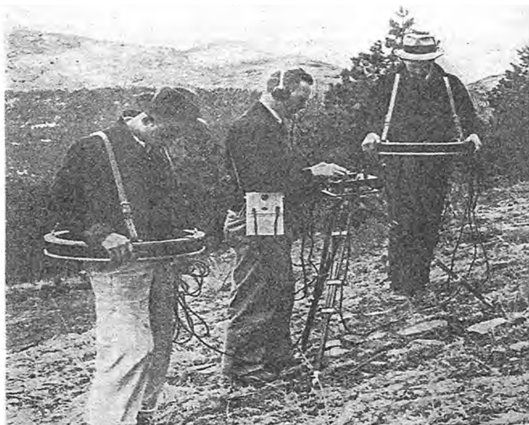
Fig. 29 - Geophysicists operating on the field with the amplitude electromagnetic method (after Heiland, 1940).
