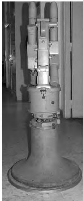
Fig. 3 - The Askania torsion balance with two-tilted beam, coupled to reduce measurement time. From the bottom: the support pedestal; the cylindrical apparatus that allows automatic rotation through a clockwork set-up for a series of prearranged orientations for measurements. At the top two opposing balances coupled with the central part where the transmission of bright rays occurs, the beam deviations are recorded onto a photographic plate. The height of the tool was 130 cm.
