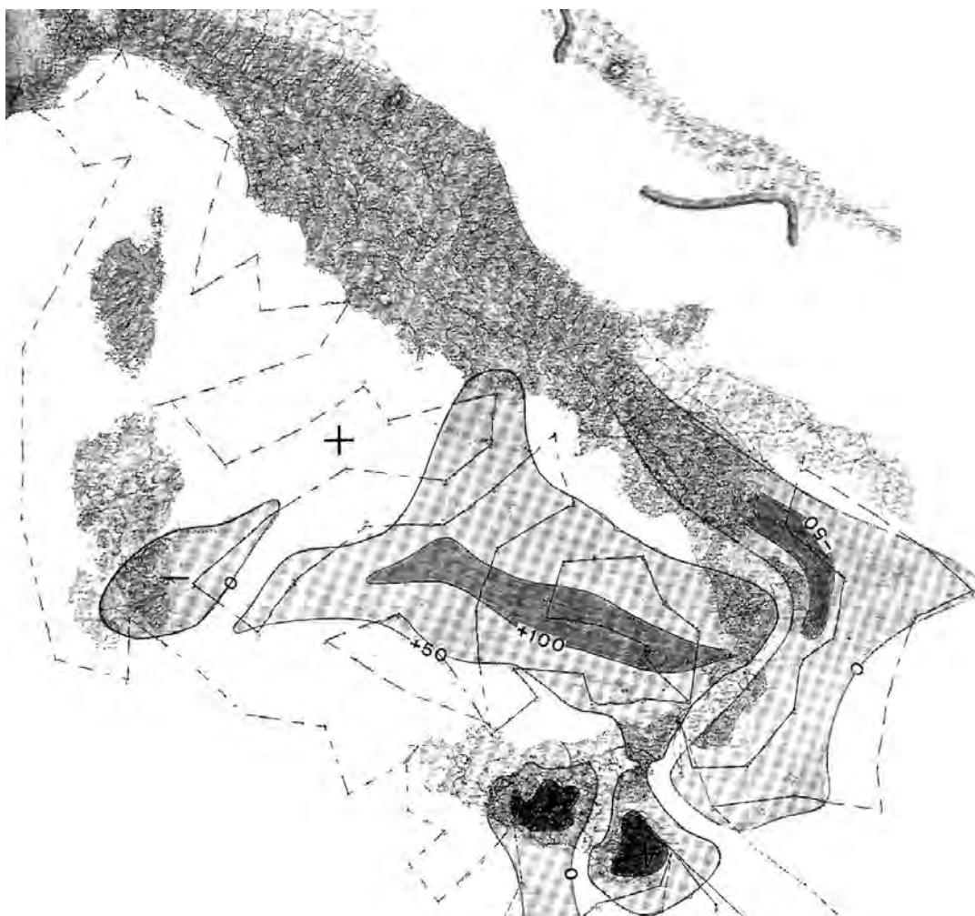
Fig. 6 - Hayford isostatic anomalies in the south Tyrrhenian and Ionian seas determined from gravity measurements performed with Vening Meinesz apparatus mounted in the Italian submarine V. Pisani (after Cassinis, 1934).
