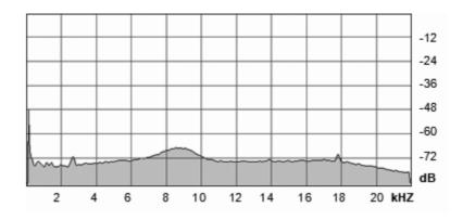
Fig. 2 - Spectrum of 2 seconds of the signal recorded in the laboratory during the compression of a sample of calcare massiccio (massive limestone). Note the hump in the frequency range 7 - 10 kHz with a peak of 6 dB above the noise level.
