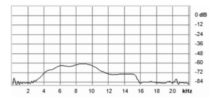
Fig. 6 - Residual spectrum of the 20 seconds of recording with a peak of 24 db above the noise level after subtracting the background noise. This figure represents the difference of the recorded signal after subtracting that of the noise.
