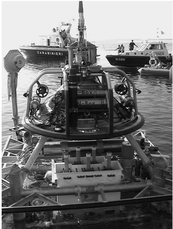
Fig. 1 - The whole GEOSTAR frame; the mobile docker, the bottom station and one of the two booming arms.
