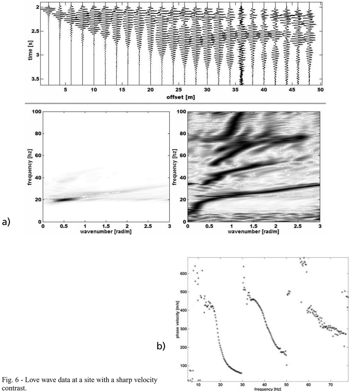
Fig. 6 - Love wave data at a site with a sharp velocity contrast.
