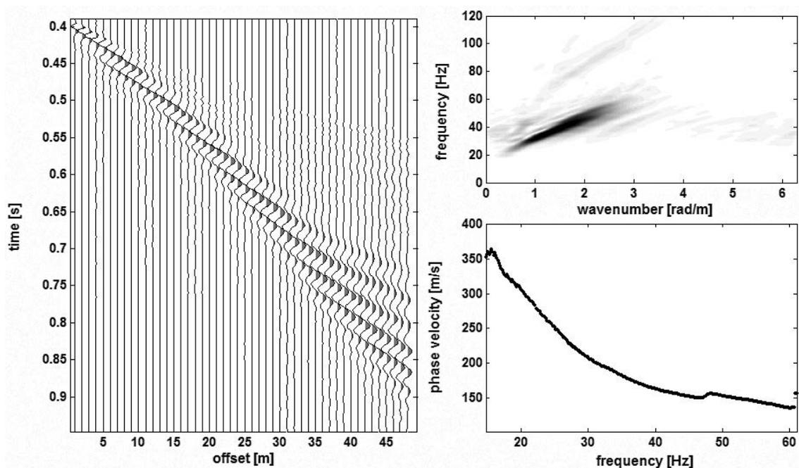
Fig. 3 - Example of processing of Love waves: the seismogram, the f-k spectrum, and the dispersion curve.
