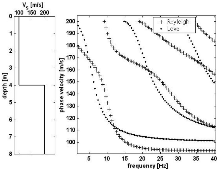
Fig. 9 - Comparison of Rayleigh and Love dispersion without anisotropy: synthetic data.
