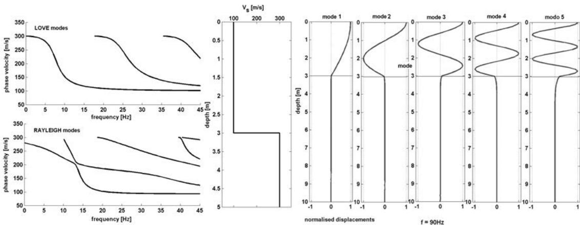
Fig. 2 - For a simple 2 layer model the modal curves of both Rayleigh and Love waves are computed (left) and the displacements with depth at a single frequency for the first 5 Love modes (right).
