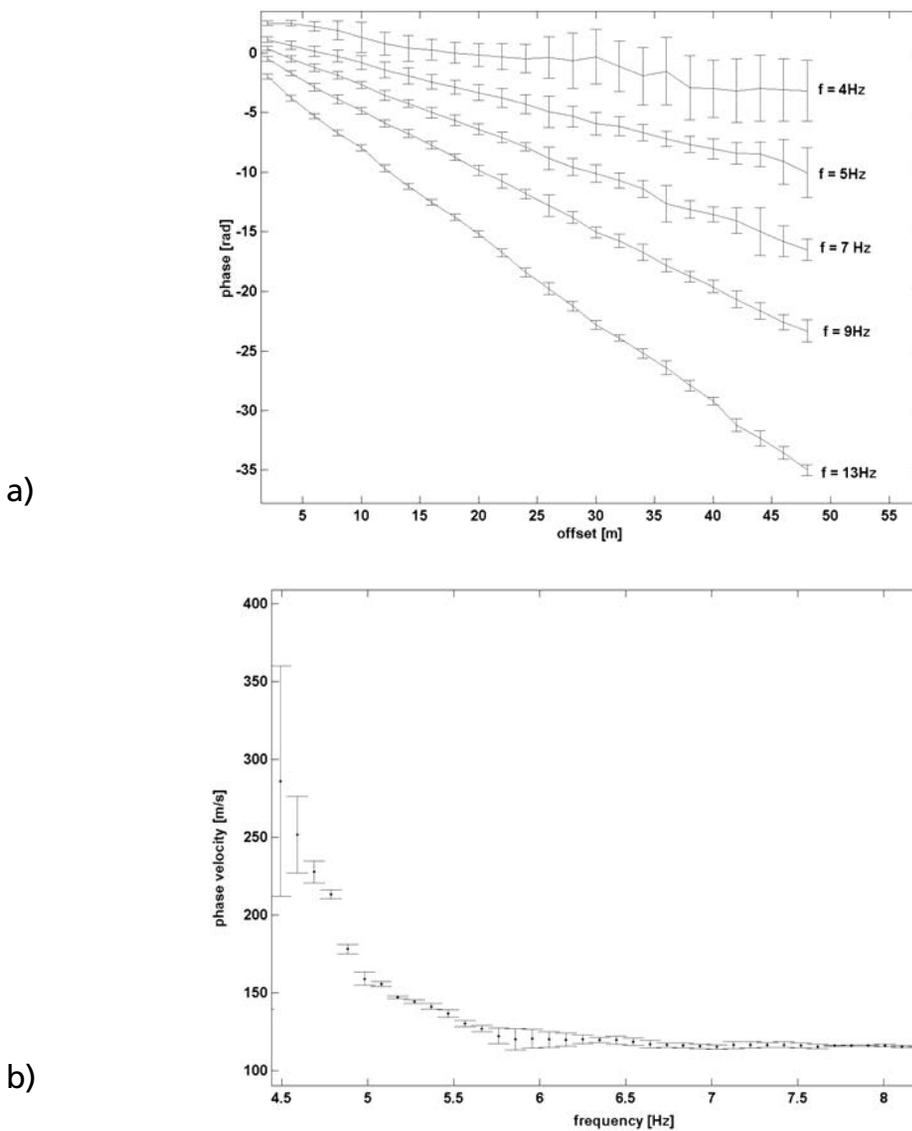
Fig. 4 - The experimental unwrapped phases at different frequencies as a function of the offset (a) are used for a weighted estimate of the wavenumbers. A linearity test is performed, then the phase velocity can be computed (b).
