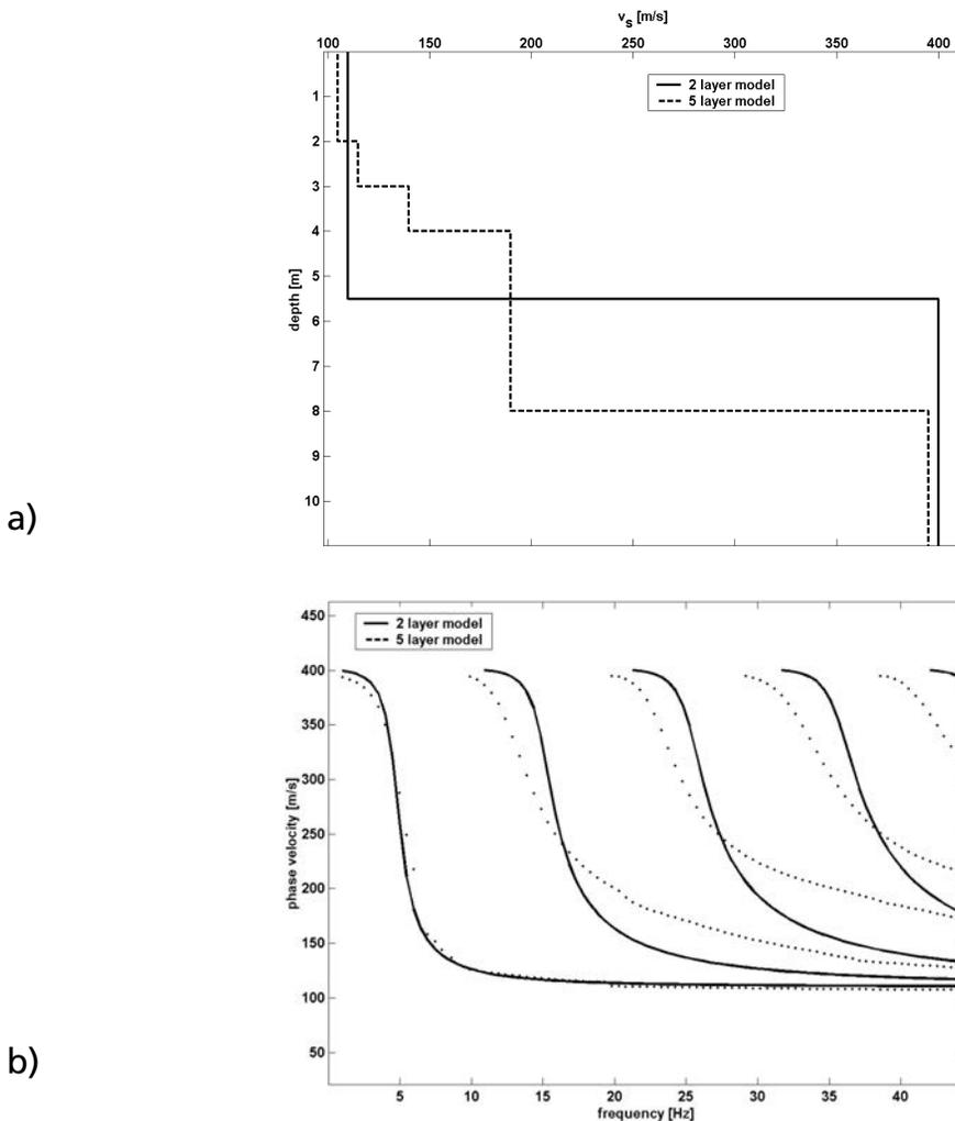
Fig. 5 - Two simple models (a) and their modal curves (b). In the inversion of the first mode the two models can be considered equivalent, while not for higher modes.
