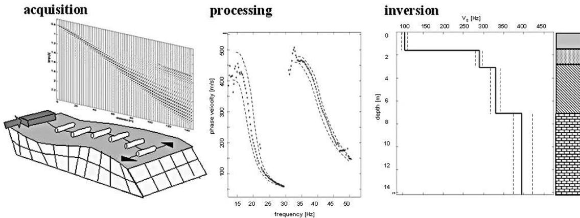
Fig. 1 - The three steps of the LWM over a real data set.
