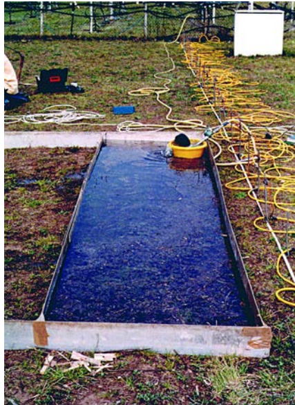
Fig. 1 - Picture of the experimental set-up for infiltration test.
