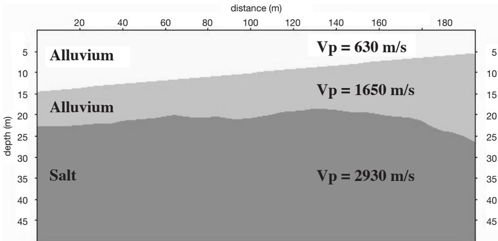
**Fig. 6** - Depth section along the refraction line located in the vicinity of the sinkhole of Fig. 5.
