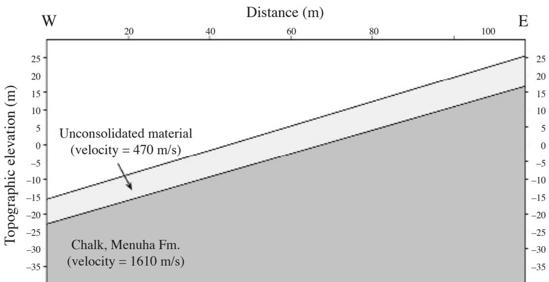
Fig. 8 - Depth section along the refraction line located on top of the Masada spur (Fig. 7).
