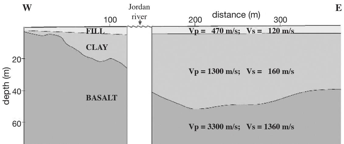
Fig. 9 - Depth section along the P- and S-wave refraction line shot along the route of a projected bridge across the Jordan river.
