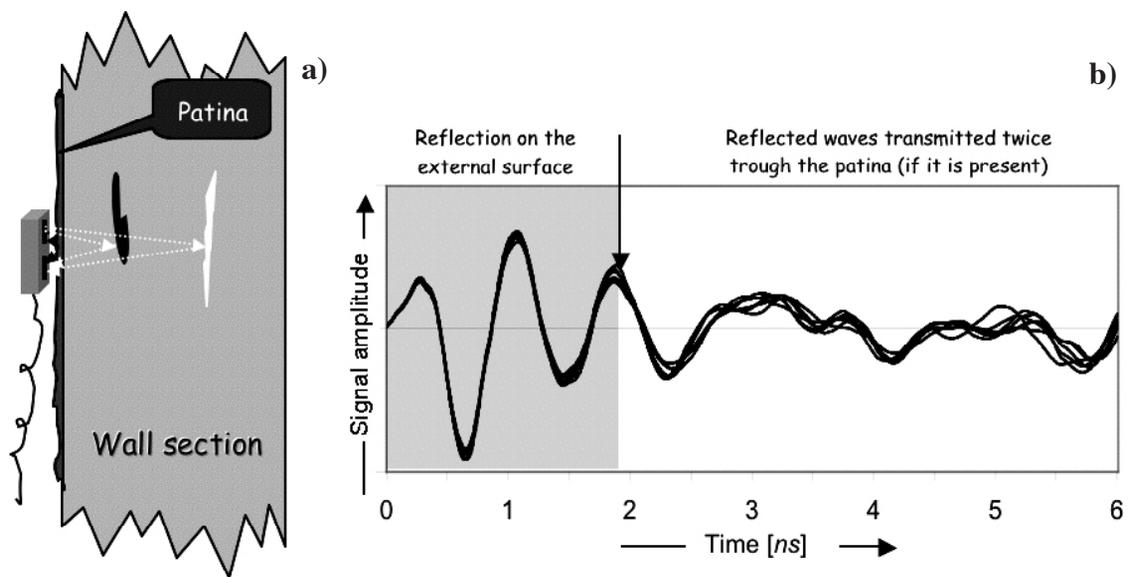
**Fig. 4** - a) Sketch of typical GPR acquisition along the surface of the wall using semi-transmission techniques. b) Traces of GPR signals (site A) showing the shape of first arrivals (gray zone) and that of later arrivals (about 2 ns delay). These, in presence of an external patina, cross twice the patina layer.
