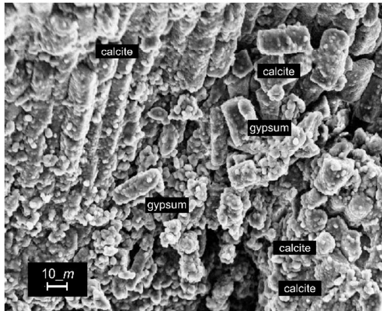
**Fig. 8** - SEM microphotograph of a patina in site B. Notice loss of cohesion of calcite and overall growth of gypsum. Reflection on the external surface.
