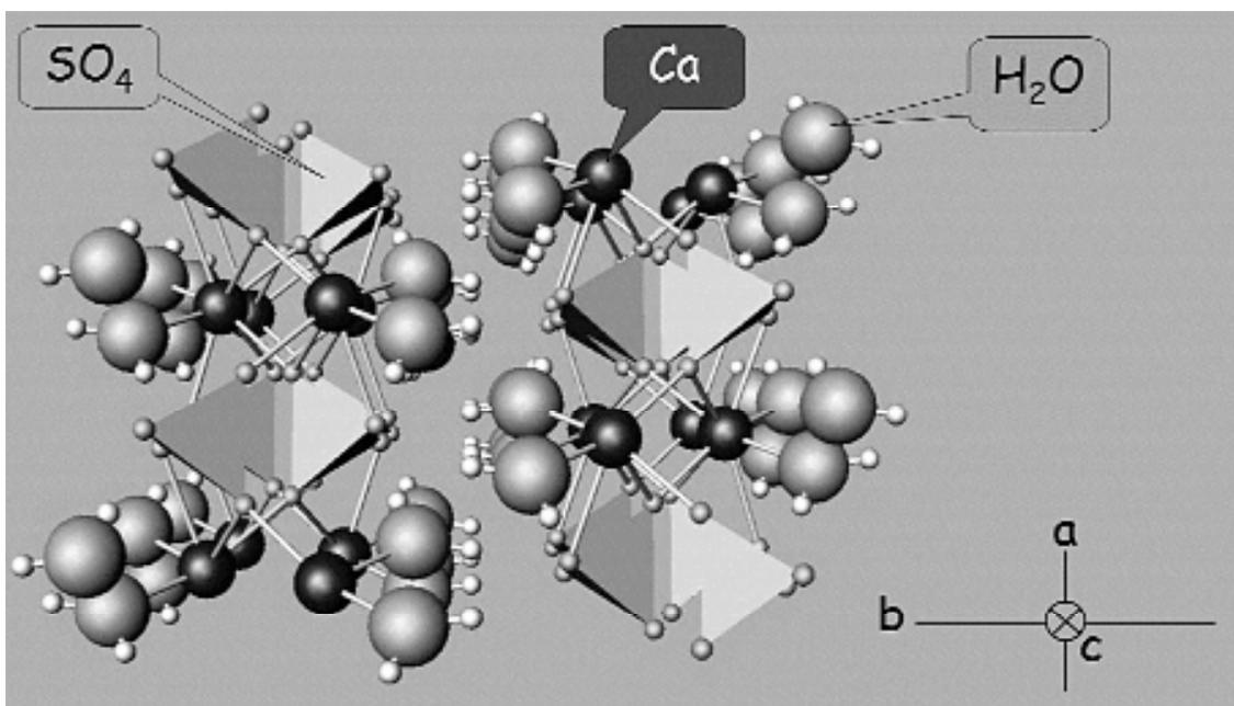
Fig. 1 - Selected view of the crystal structure of gypsum with reference to crystal axes.
