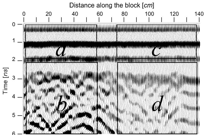
**Fig. 3** - Typical file recorded in site A. The profile crosses the separation between patina-free and patina-rich areas at about 65 cm. The spectral responses of the parts of signals contained in frames *a*, *b*, *c* and *d* are, respectively, presented in Fig. 5.
