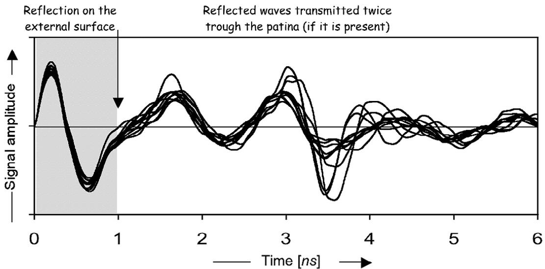
**Fig. 6** - Typical signals recorded at site B. Notice that the two-way travel time of the waves reflected inside the wall appears to be shorter than in fig. 4b. This delay, on average, is estimated at about 0.8 - 1 ns.
