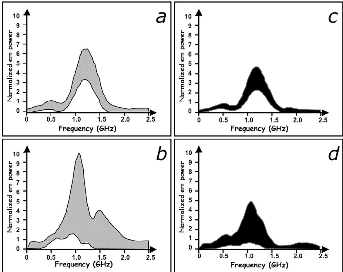
Fig. 5 - Spectral responses of parts of signals presented in Fig. 3. Spectra *a* and *b* refer to patina-free areas while *c* and *d* to patina-rich areas. Notice damping of amplitude in *d*, especially in the 1.3 - 2.0 GHz frequency range.
