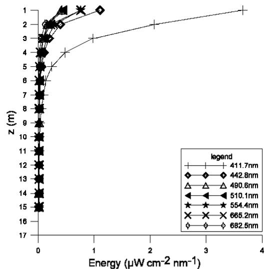
Fig. 8 - Energy attenuation in the seven wavelengths for light emitted by 400 Watt metallic iodide lamp.
