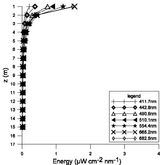
Fig. 7 - Energy attenuation in the seven wavelengths for light emitted by 1000 Watt incandescence lamp.
