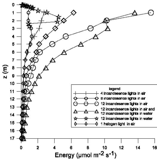
Fig. 1 - Energies recorded close to the fishing vessel indicated that light intensity decreased exponentially along the water column.
