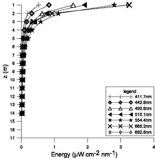
Fig. 5 - Energy attenuation in the seven wavelengths for light emitted by 1500 Watt halogen lamp.
