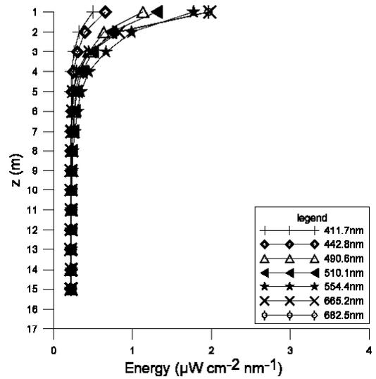
Fig. 6 - Energy attenuation in the seven wavelengths for light emitted by 1000 Watt halogen lamp.
