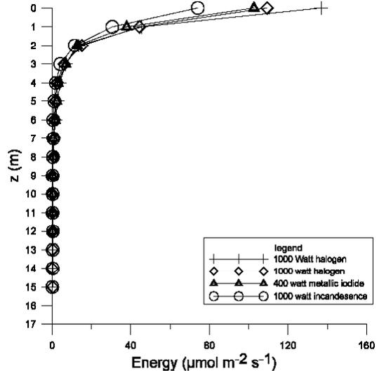
Fig. 4 - General pattern of the vertical profiles of light attenuation in the PAR range for four different lamps.
