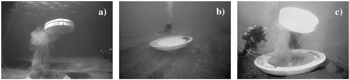
Fig. 3 - BARNY Sentinel emergency recovery: (a) fire of second releaser; (b) platform inverted; (c) fire of second releaser with platform inverted.
