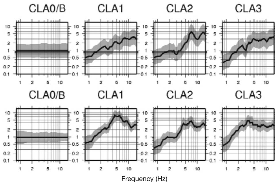
**Fig. 6** - Spectral ratios determined for stations Cla0/B, Cla1, Cla2 and Cla3 from year 2000 data subset. Diagrams (with respect to the reference site Cla0/B) displaying vertical component ratios above, horizontal ones illustrated below. The grey area shows standard deviation.
