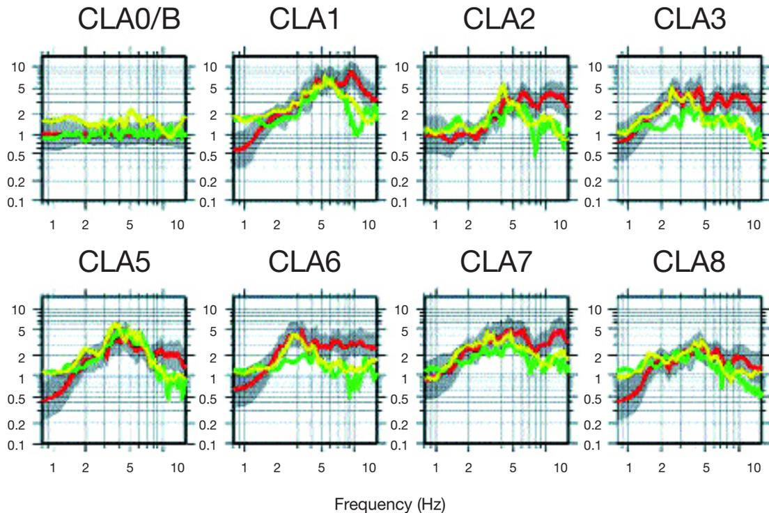
**Fig. 10** - Graphic comparison of results from the different spectral analyses performed in our study: spectral ratio (red), receiver function (yellow), Nakamura (green). In grey is represented the confidence limit equal to  $\pm \delta$ .
