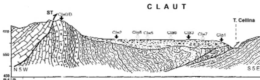
**Fig. 3** - Geological cross-section striking through the village of Claut. Location of seismic stations: Lennartz MarsLite data loggers (Black arrows); Nanometrics Orion data loggers (white arrows).
