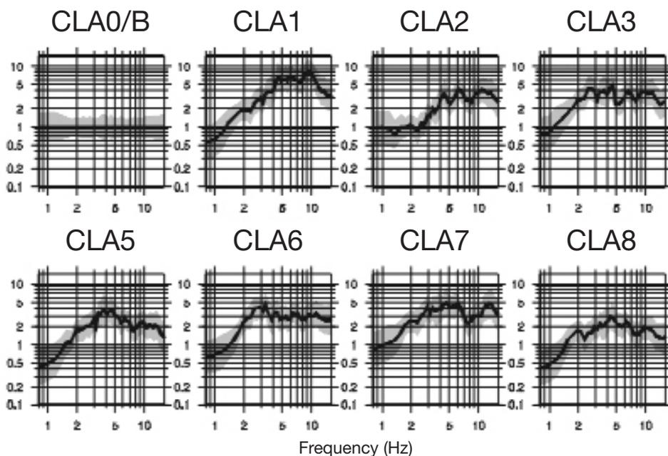
**Fig. 7** - Spectral ratios (with respect to the reference site Cla0/B; horizontal components illustrated only) computed for stations Cla0/B, Cla1, Cla2, Cla3, Cla5, Cla6, Cla7 and Cla8 for 2001 data subset. The grey area shows standard deviation.
