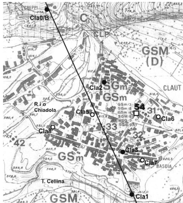
**Fig. 2** - Map of Claut village: open square (54) geomechanical survey and correspondent litostatigraphic column found; (31-32-33-42) V.E.S.; Lennartz MarsLite data loggers (black circle); Nanometrics Orion data loggers (open circles).
