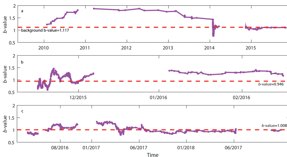
Fig. 10 - Temporal variation of b -value throughout the 2015 sequence, related to the aftershock zone depicted in Fig. 9. The red dashed lines represent the b -value estimation for the entire subset. The magenta lines are derived by moving the window of N = 50 events through the catalogue event by event and plotting the data at the end of the considered time interval. The computations refer to panel: a) the long-term background seismicity, covering the period from 2008 until the last event preceding the M_w 6.5 earthquake; b) the period related to the aftershock sequence from 17/11/2015 until 31/03/2016; c) the time interval after the aftershock sequence.
