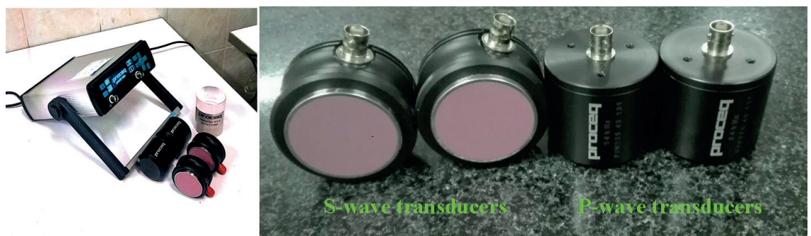
Fig. 3 - Pundit Lab device and P- and S-wave transducers.
