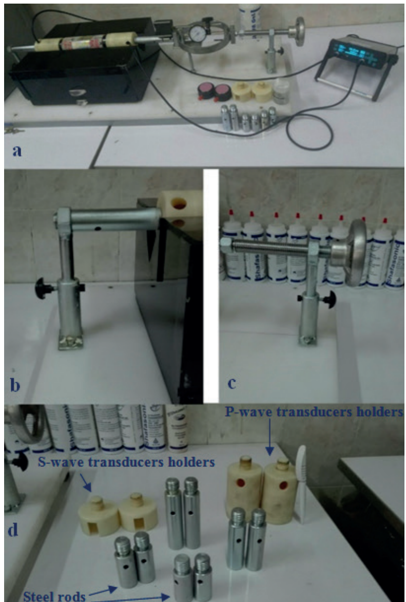
Fig. 2 - The ultrasonic apparatus prepared for testing (a), height adjustment screw (b), rotary handle (c), the steel rods with different lengths and transducer holders (d).
