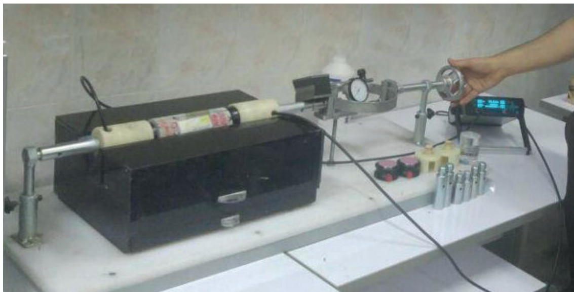
Fig. 4 - Applying the required stress by rotating handle.
