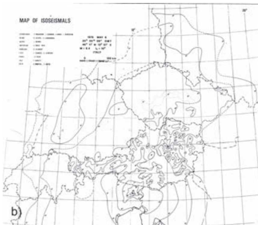
Fig. 8 - Joint macroseismic maps of the 1976 Friuli main shock after Kárník et al. (1978, left) and after Procházková and Kárník (1978). In Fig. 8b (right), the southern part is omitted. Both maps refer to the same basic map, but have a slightly different layout.
