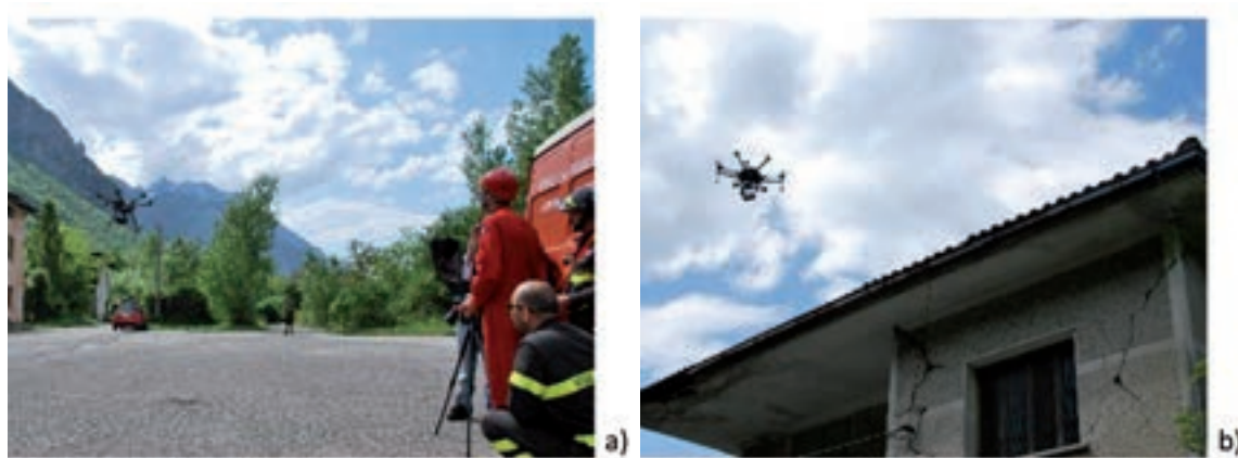
Fig. 11 - Use of drones to assess the safety conditions of buildings damaged by the earthquake: a) the drone is piloted from a remote safe place; b) the drone investigates an area not visible from the ground.
