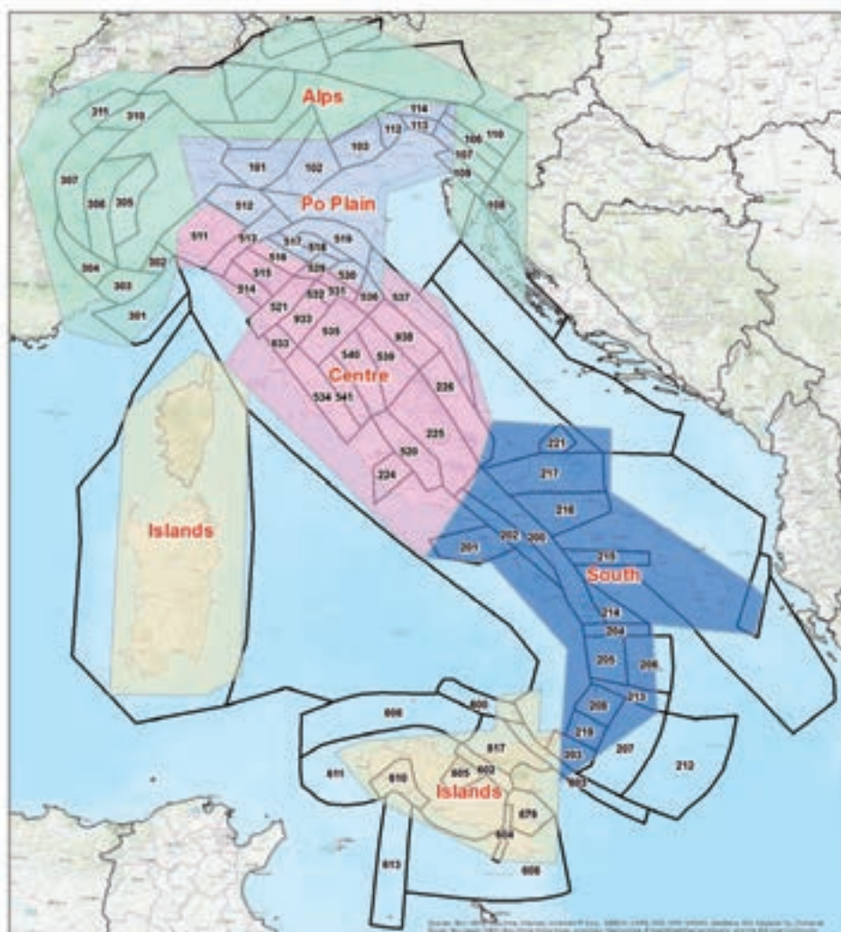
Fig. 4 - The A1 zonation (boxes with black perimeter) and macro areas (coloured polygons) identifying homogeneous regions for the assessment of completeness.
