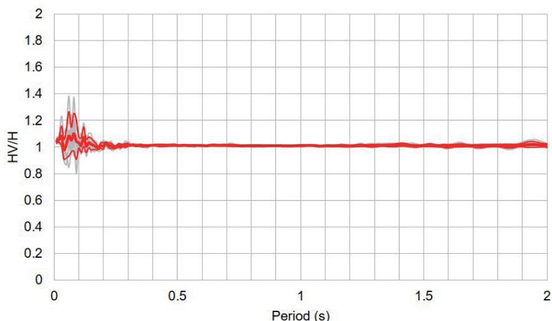
Fig. 4 - HV/H ratios at the site of Cascia (Fig. 1). Grey lines indicate HV/H ratios relative to each single accelerometric time history. Continuous thick red line represents the median of the HV/H ratios and the two thin red lines respectively represent 84<sup>th</sup> and 16<sup>th</sup> percentiles.
