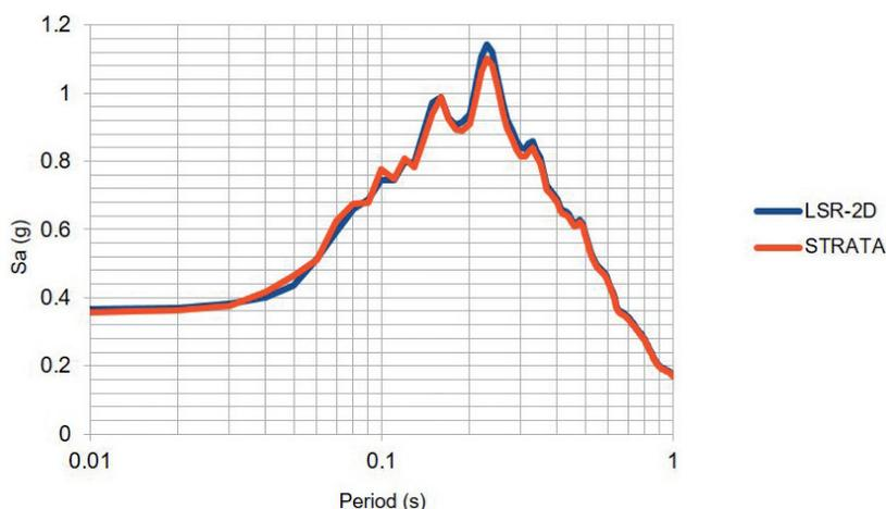
Fig. 3 - Comparison between outcomes of STRATA and LSR-2D codes for the same subsoil configuration. In the plot, average elastic response spectra ( $S_a$ ) obtained for the same horizontal input motion by the two codes LSR-2D and STRATA by considering the 7 accelerograms at the Gildone site (Fig. 1).
