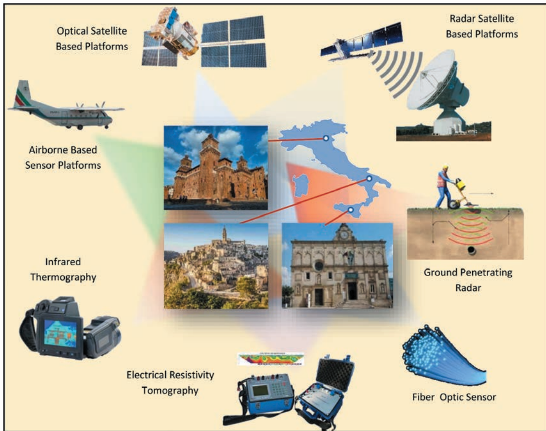
Fig. 9 - Map of the test-sites and simplified diagram illustrating the geophysical monitoring strategy approach adopted by the CLARA project. The approach combines satellite and ground-based observations, geophysical tomographic methods, new sensors with multi-resolution in space and time domains.
