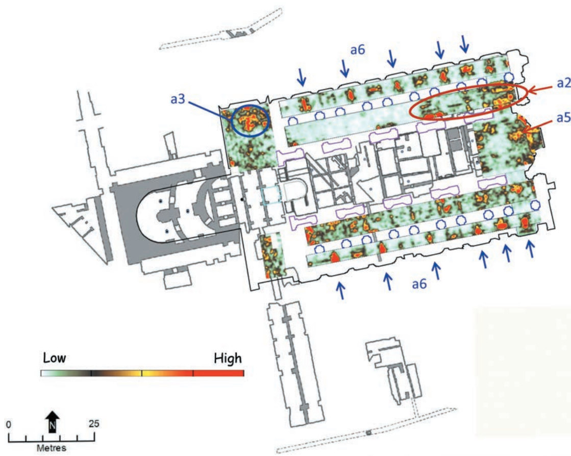
Fig. 11 - St. John Lateran Basilica. GPR 400 MHz, slices at the estimated depth of 4.20 m.
