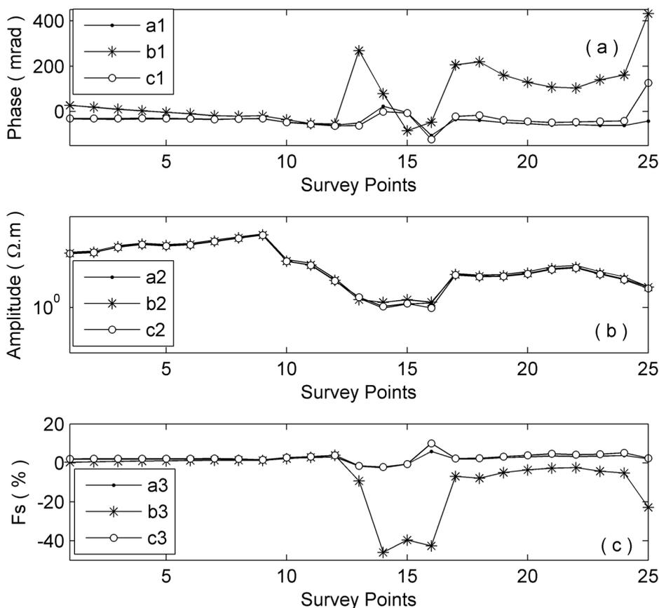
Fig. 6 - a) a1: phase at 0.01 Hz; b1: phase at 1 Hz; c1: relative phase at 1 Hz. b) a2: amplitude at 0.01 Hz; b2: amplitude at 1 Hz; c2: corrected amplitude at 1 Hz. c) a3: polarizability at 0.01 Hz; b3: polarizability at 1 Hz; c3: polarizability at 1 Hz.
