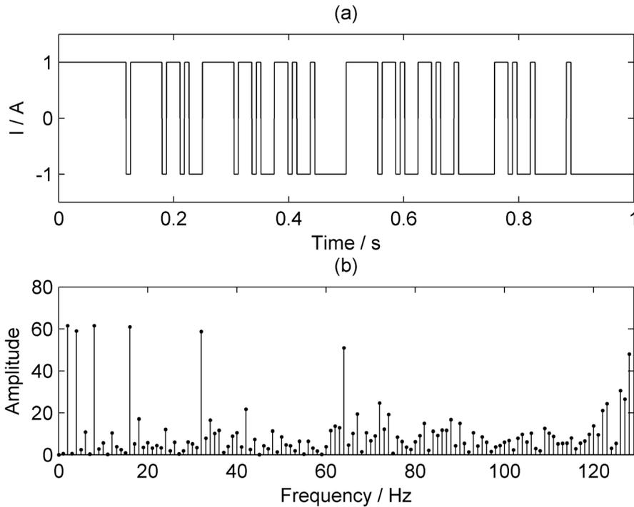
Fig. 2 -  $2^7$ -sequence current: a) waveform corresponds to one period; b) amplitude spectrum.
