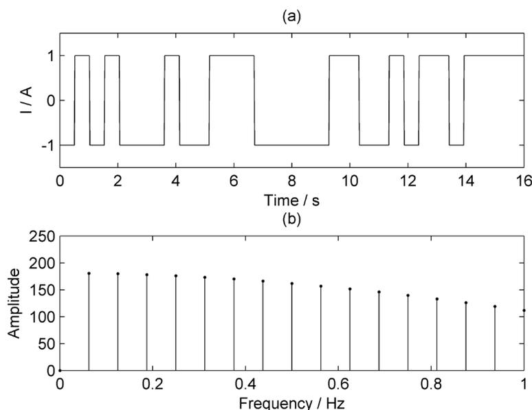
Fig. 1 - 5-order m-sequence current: a) waveform corresponds to one period, b) amplitude spectrum at 0 - 1 Hz.
