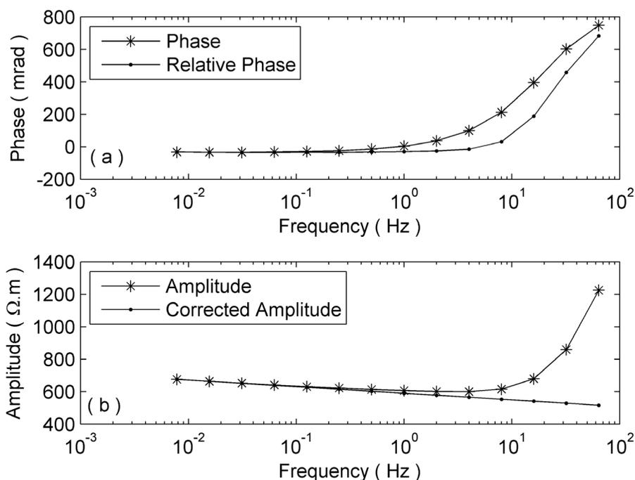
Fig. 5 - Phase spectrum and amplitude spectrum before and after correction.
