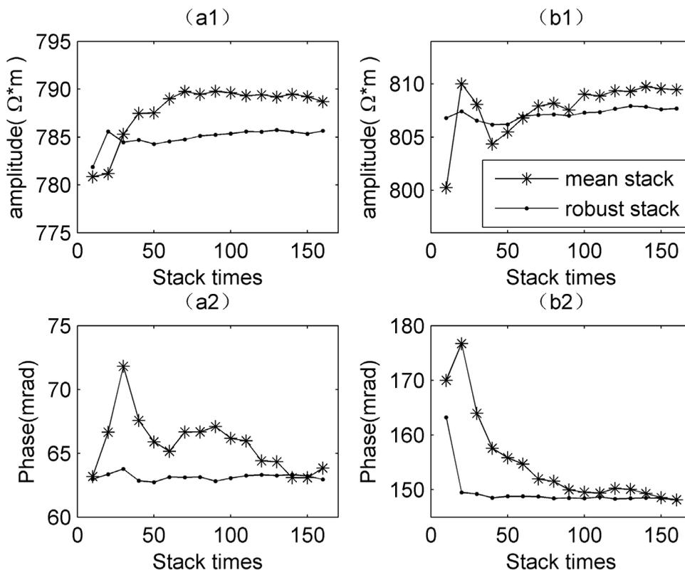
Fig. 3 - Convergence of complex resistivity with stack times for different stacking methods: a1) amplitude at 5/16 Hz; a2) phase at 5/16 Hz; b1) amplitude at 12/16 Hz; b2) phase at 12/16 Hz.
