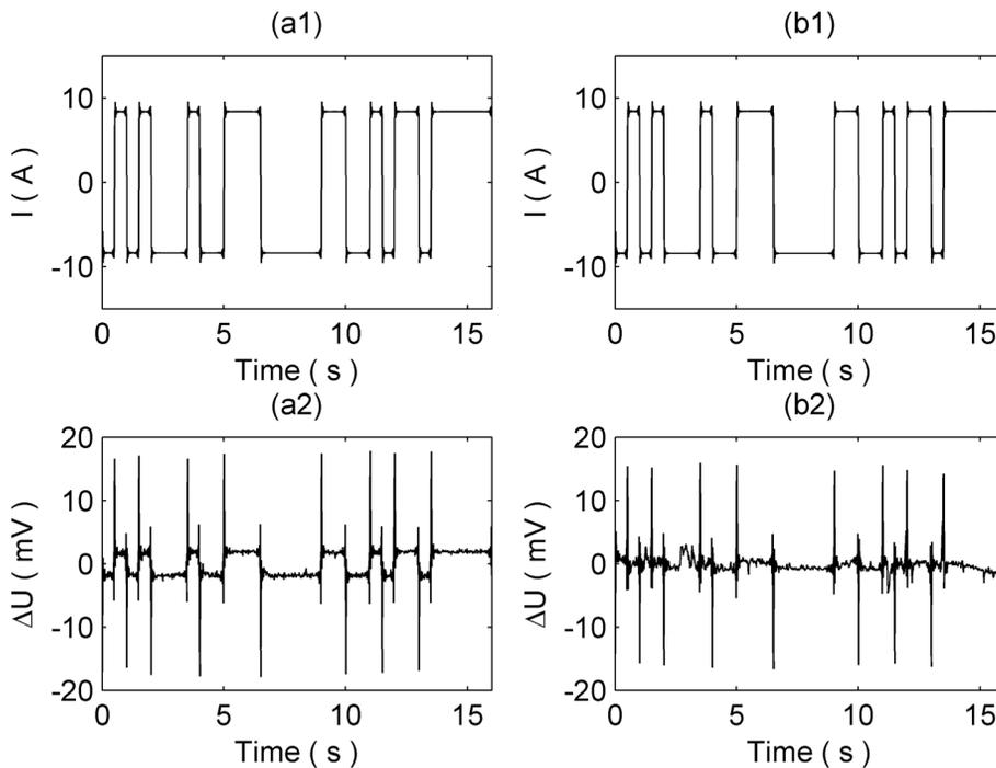
Fig. 4 - a1) current signal in the period showing coherence of 0.59; a2) potential signal in the period showing coherence of 0.59; b1) current signal in the period showing coherence of 0.01; b2) potential signal in the period showing coherence of 0.01.
