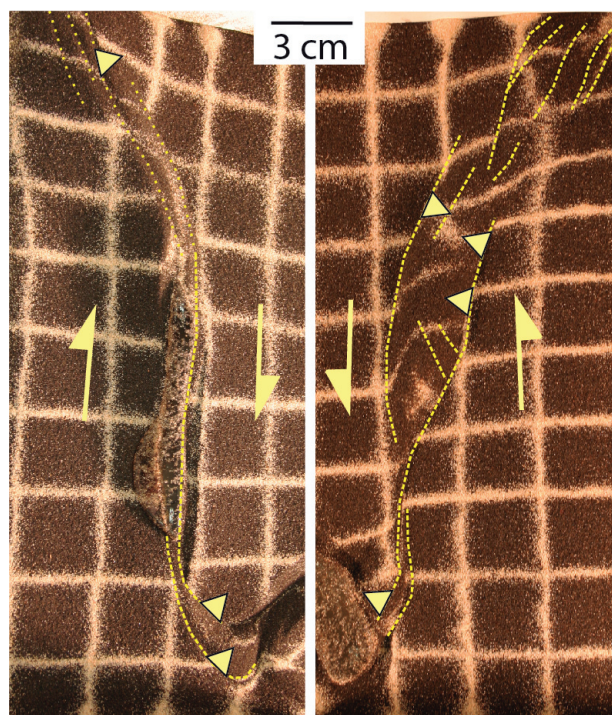
Fig. 7 - Detailed photographs of the strike-slip fault zones developed at both laterals of Experiment 2.
