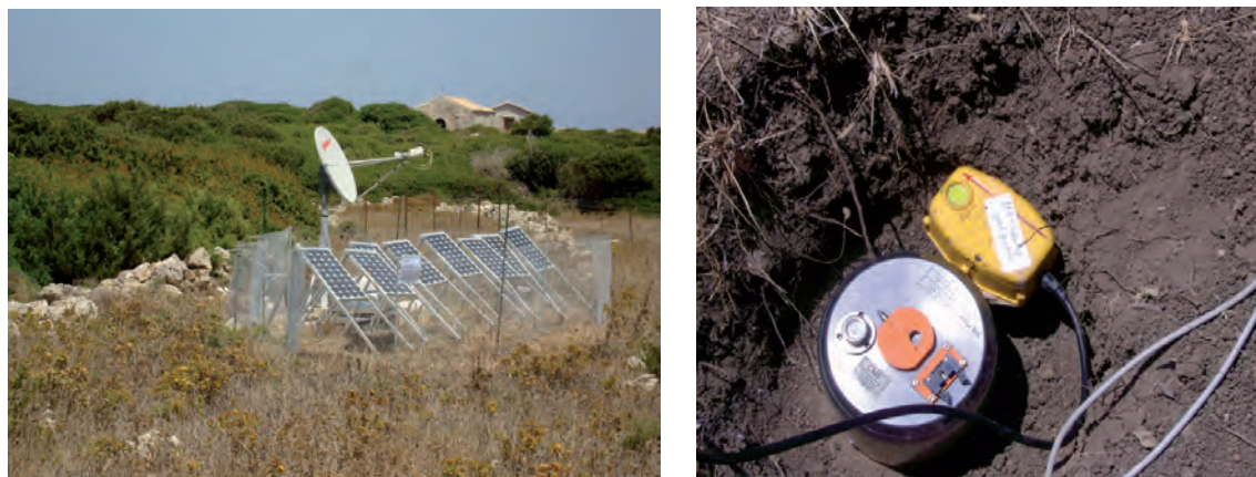
Fig. 10 - The seismic station on the Strophades Island (left). Broadband and 4.5 Hz geophone (right).
