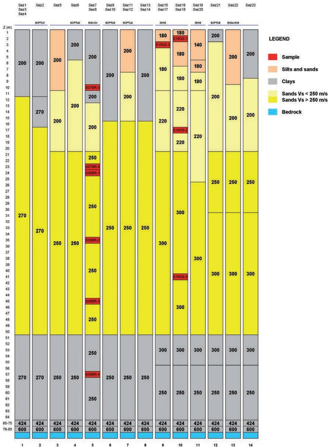
Fig. 8 - Seismo-stratigraphic sequences for the macro-area Guastalla: the thickness of each layer is given on the left (m), and the shear wave velocity values are given on each layer of the column (m/s).
