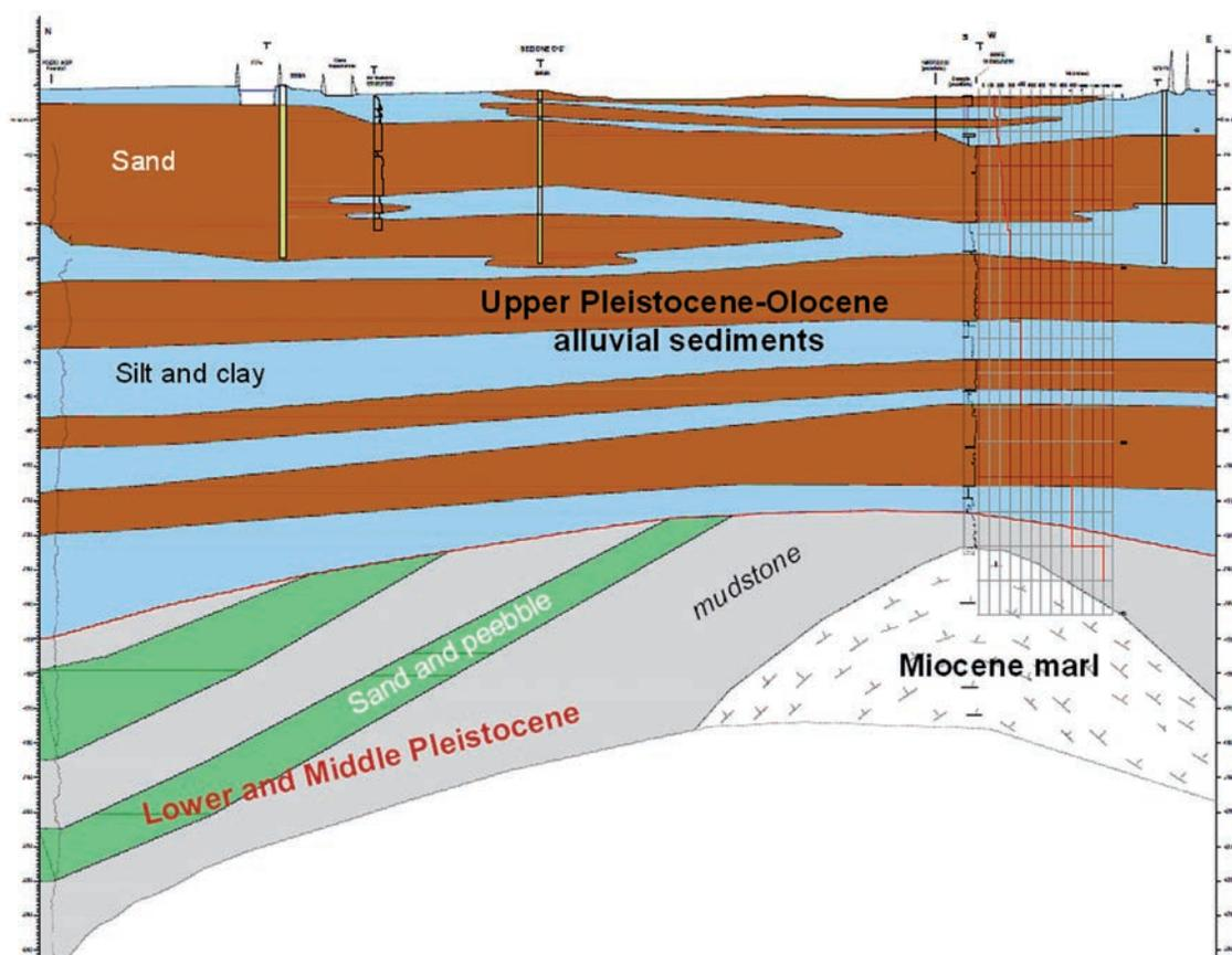
Fig. 5 - Geological model of the Ferrara area; in the figure the values of the bore-hole, CH and CPT are reported.
