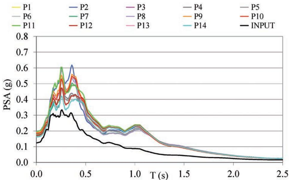
Fig. 10 - Curves of the average acceleration response spectra for the analyzed 14 seismo-stratigraphic sequences.
