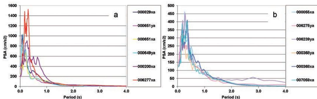
Fig. 6 - Acceleration response spectra for the macro-area of Ferrara (a), macroseismic hazard, and for the macro-area of Guastalla (b), standard hazard.
