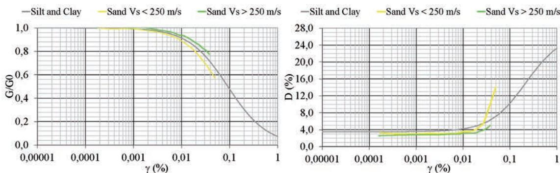
Fig. 9 - Decay curves for the different geologic units: behaviour of the  $G/G_0$  and  $D$  curves with the shear strain.
