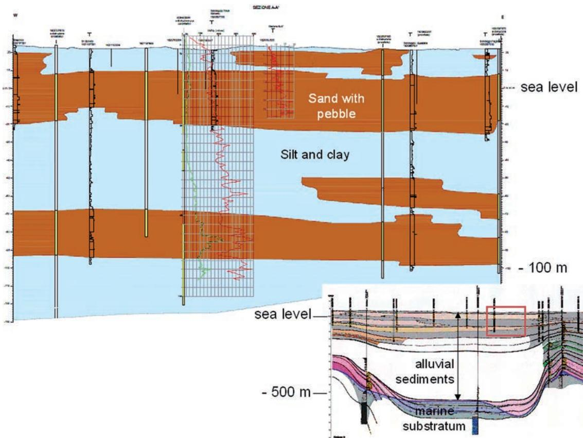
Fig. 4 - Geological model of the western sector; in the figure the values of the bore-hole, CH and CPT are reported.
