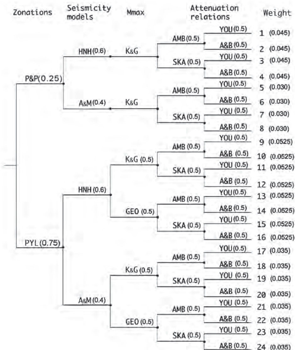
Fig. 3 - Logic tree used for PSHA of the Pylos broader area (see the text for the acronyms).
