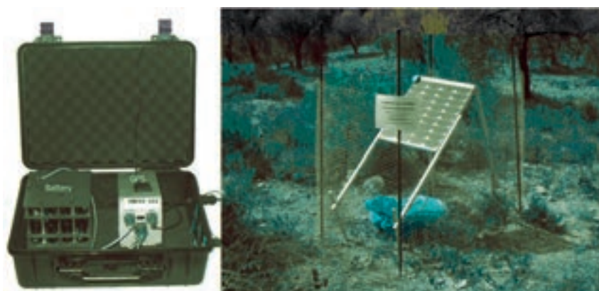
Fig. 3 - The GeoPro stand alone seismic station contained in a waterproof plastic box (left). The station has 6 channels and can record for 1 month on alkaline D-size batteries or continuously with solar panels (right).
