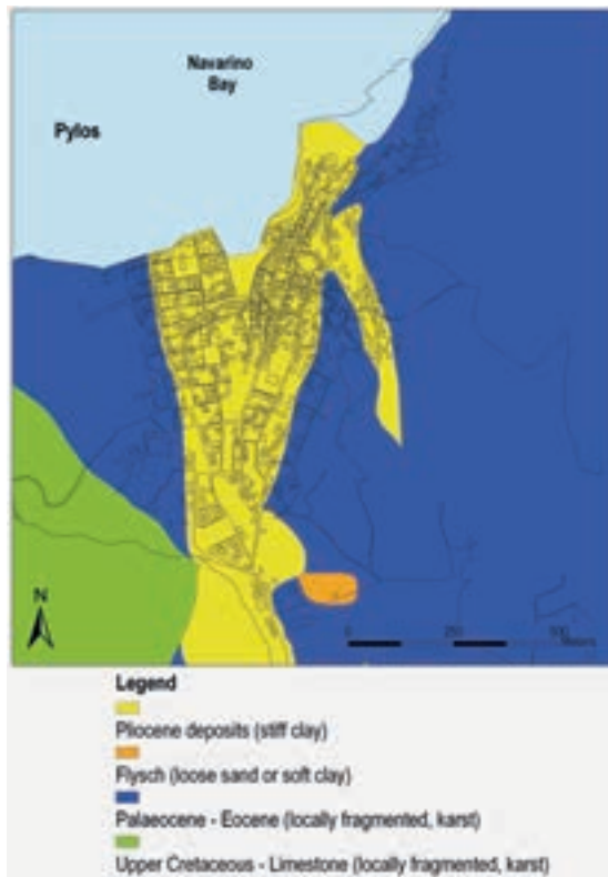
Fig. 4 - Geotechnical map of Pylos town overlaid on the town plan (source: EPPO, 1987).
