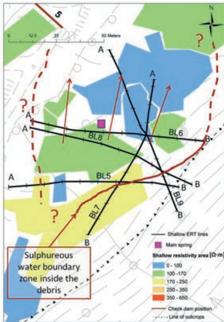
Fig. 5 - Location map of the shallow ERT profiles (2 m spacing) in the main spring area. The resistivity areas from FDEM survey are also shown (Fig. 4), superimposed on the technical map.
