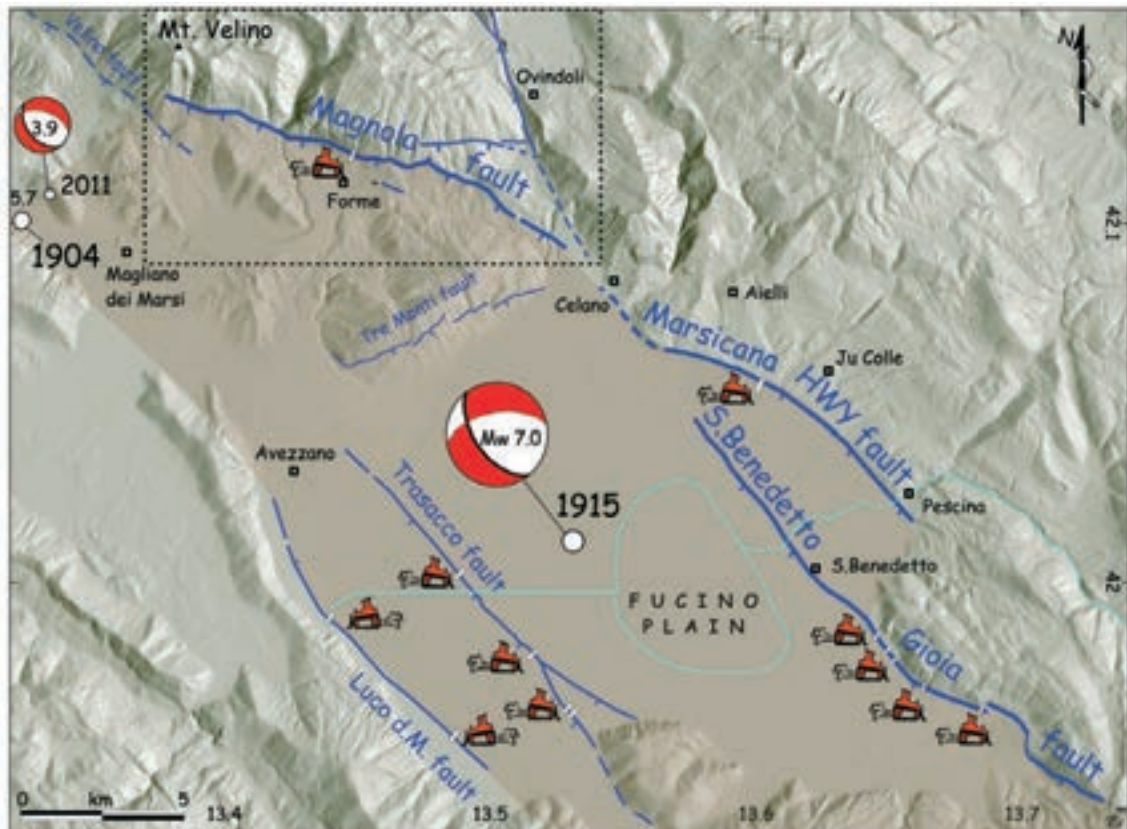
Fig. 2 - Expanded digital terrain model from Fig. 1 of the Fucino fault system, which was the structure responsible for the M_w \sim 7 earthquakes of 1915, 508 AD, and many previous paleoseismic events. The main faults bounding at the NE of the Fucino basin are in bold blue (the Magnola, Marsican Highway, and Gioia dei Marsi-San Benedetto dei Marsi faults). The main synthetic (Trasacco), antithetic (Luco dei Marsi) and transversal (Tre Monti) faults are in blue. Note at the NW tip of the Magnola fault the epicentres of the M_w 5.7, 1904 and the M_w 3.9, 2011 earthquakes. The darker area fits the rough surface projection of the in-depth seismogenetic structure. Bulldozers are paleoseismological sites where paleoearthquakes have been identified [see text and Galli et al. (2008)]. Focal mechanisms are from Gasparini et al. (1985) and SLU-EC (2011). Dashed rectangle shows area of Fig. 5.
