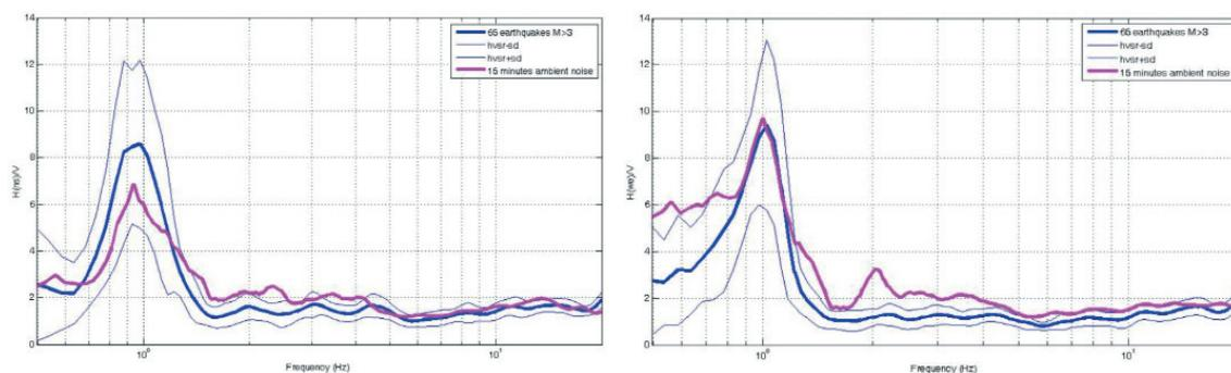
Fig. 8 - HVSR curves for the two components (N-S on the left and W-E on the right) of Castelnuovo by 65 earthquakes with  $M_L > 3$  and 15 minutes of ambient noise recordings.
