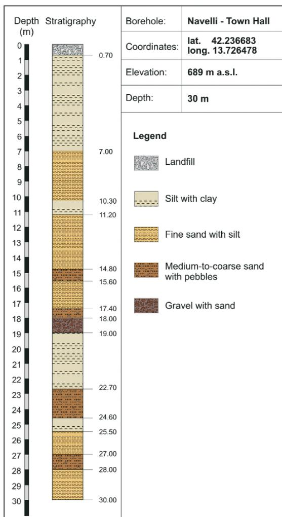
Fig. 3 - Stratigraphic log of the geological borehole which has been drilled in the foundation soil of the town hall building of Navelli.
