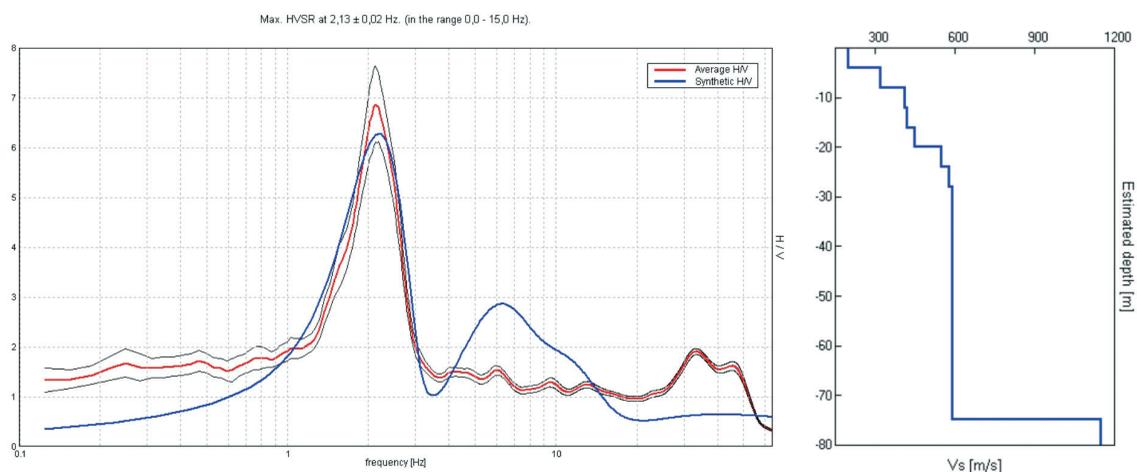
Fig. 6 - Comparison between ambient noise and synthetic HVSR curves (left) obtained at the town hall site in Navelli;  $V_s$  profile of the same site (right).
