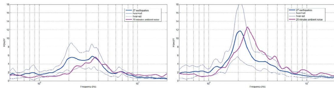
Fig. 10 - HVSR curves for the two components (N-S on the left and W-E on the right) of San Gregorio by 27 earthquakes and 20 minutes of ambient noise recordings.
