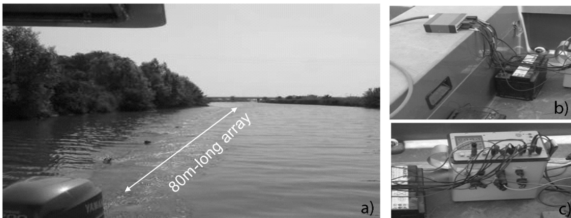
Fig. 6 - The CERT system: a) the floating marine multipolar cables with graphite electrodes, b) the energy source, c) the IRIS Syscal Pro 72 Switch georesistivity meter.
