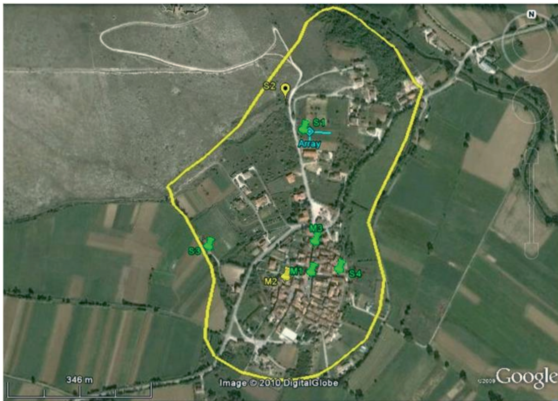
Fig. 8 - Distribution of the passive measurements (both single- and multi-station) effectuated in the area of Sant'Eusanio Forconese. The colors refer to single-station measurement quality (green: class A; yellow: class B), where the two symbols indicate the presence or not of a peak (drawing pin: type 1, i.e., presence of at least a pick; drop: type 2, i.e., no pick). The array branches are pointed out by two cyan segments.
