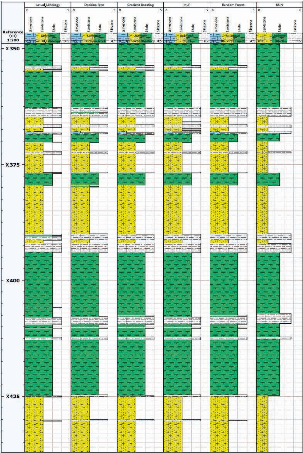
Fig. 18 - Comparison of reference and predicted lithology profiles for a representative well using different classifiers. The true lithology is shown alongside DT, GB, MLP, RF, and KNN predictions computed with identical entropy features and sliding-window settings. RF and GB exhibit the most continuous and stable boundaries, while DT and KNN show higher sensitivity to lithological transitions and greater prediction variability.
