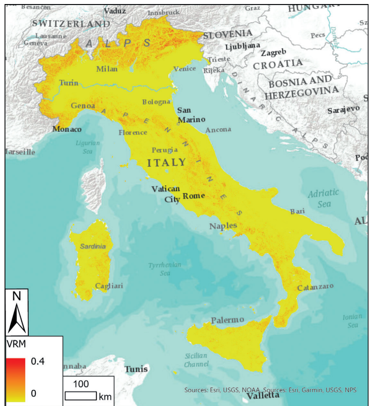
Fig. A2 - VRM map calculated with a spatial resolution of 150 m. The raster has a minimum value of 0, a maximum value of 0.4, and an average value of 0.006.
