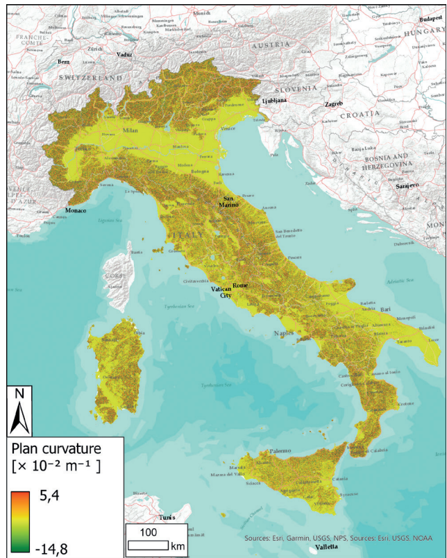
Fig. A6 - Plan curvature map calculated with a spatial resolution of 150 m. The raster has a minimum value of -14.8 \times 10^{-2} \text{ m}^{-1} , a maximum value of 5.4 \times 10^{-2} \text{ m}^{-1} , an average value of 0.005 \times 10^{-2} \text{ m}^{-1} , and a standard deviation of 0.15 \times 10^{-2} \text{ m}^{-1} .
