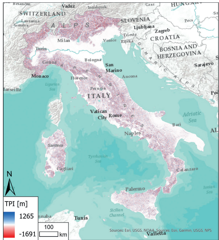
Fig. A4 – TPI map calculated with a spatial resolution of 150 m. The raster has a minimum value of -1,691 m, a maximum value of 1,265 m, and an average value of 2.52 m.
