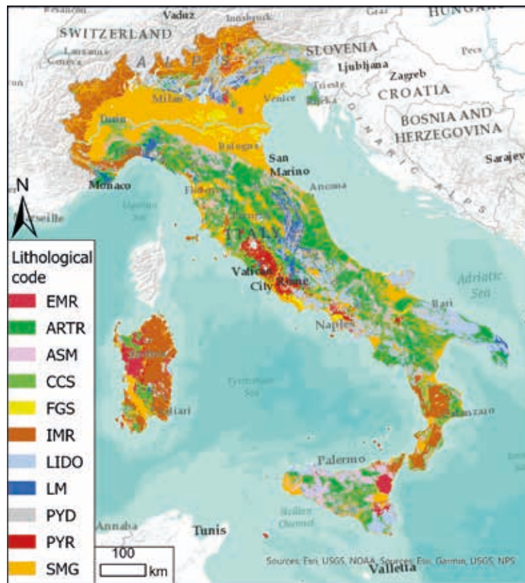
Fig. 8 - Proposed lithological classification derived from the 50 original classes of the ISPRA (2021) lithological map.
