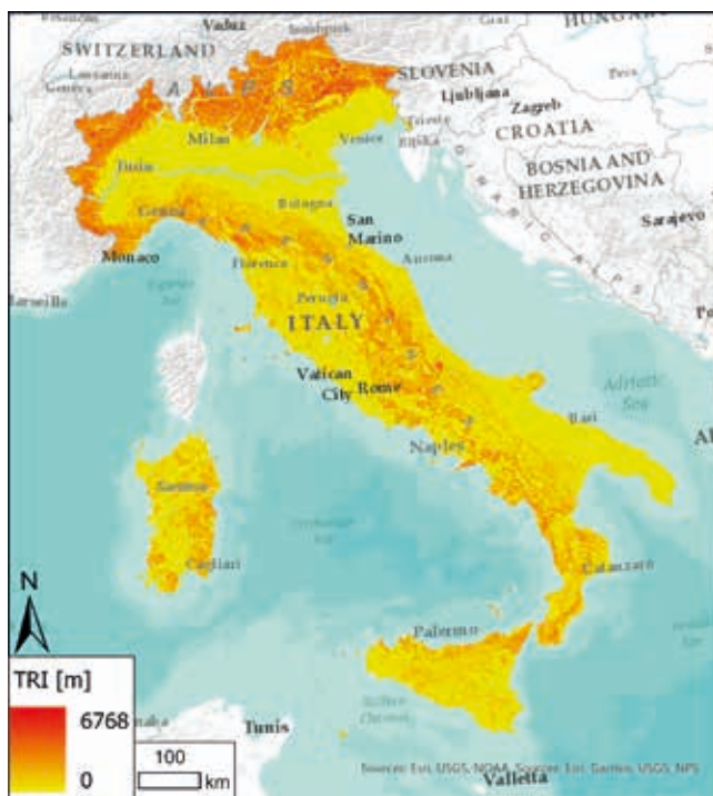
Fig. A1 - TRI map calculated with a spatial resolution of 150 m. The raster has a minimum value of 0, a maximum value of 6,768 m, and an average value of 78 m.
