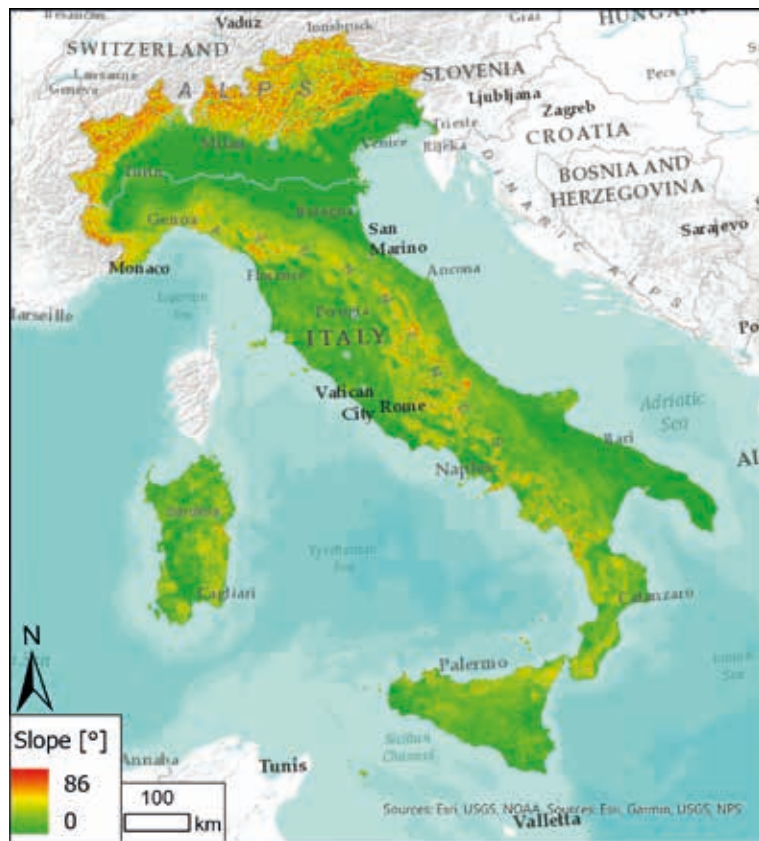
Fig. 3 - Slope map expressed in degrees and calculated with a spatial resolution of 150 m; the average value is 9.4°.
