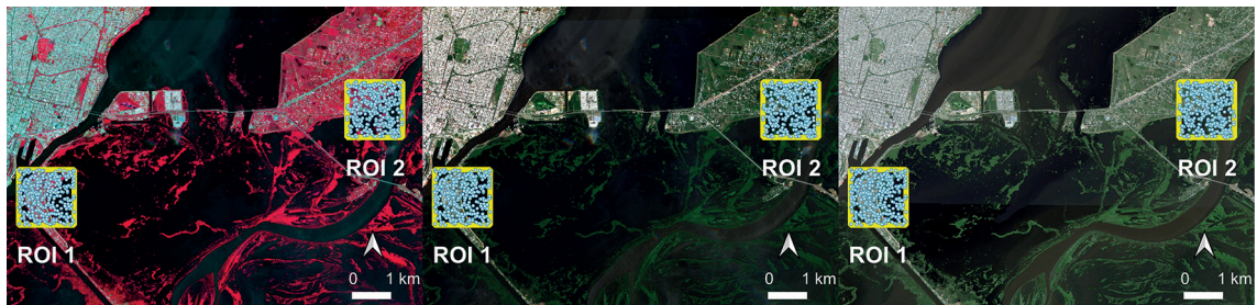
Fig. 4 - A false-colour composite (left), a natural colour composite (centre), and a Google Earth image from 14 January 2016 (right) are taken as reference images and compared with the binary image through random sampling points (cyan points) within two ROIs (yellow squares).
