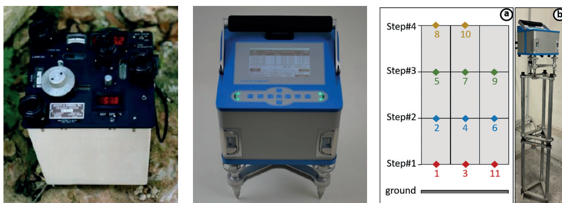
Fig. 3 - The relative gravimeters used in the frame of the project: LaCoste & Romberg, model D (left); Scintrex CG-6 (middle) both employed to measure the VGG and the gravity difference from the absolute to the auxiliary outdoor point; example of measurement scheme and tripod frame employed to measure the VGG at the absolute stations (right).
