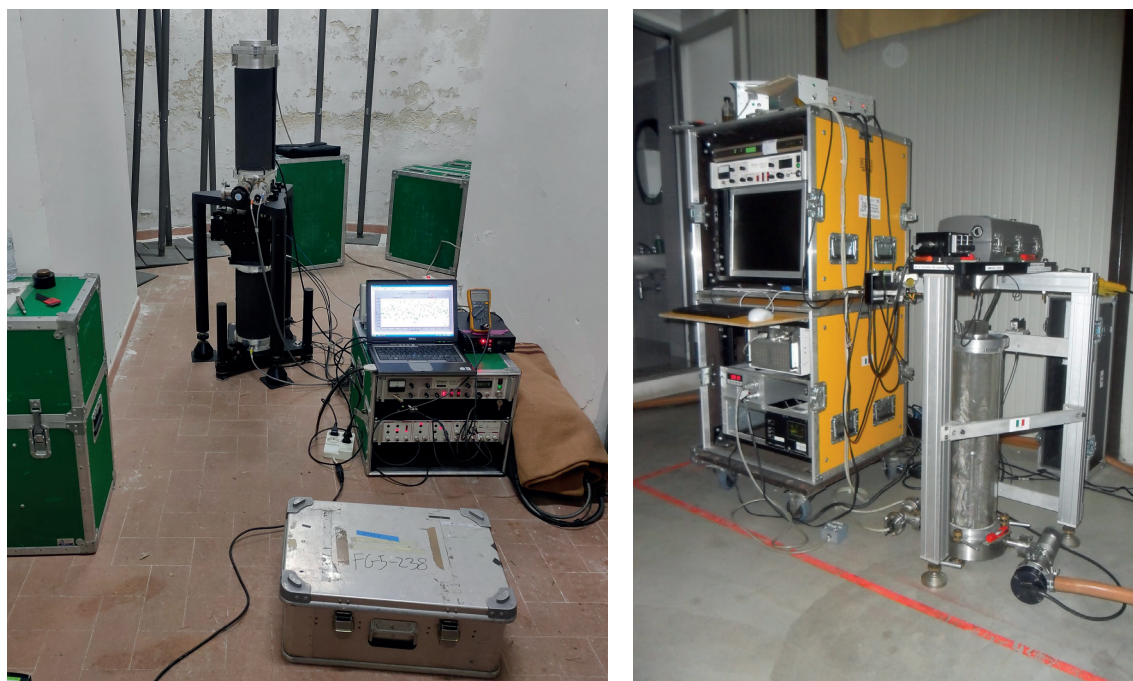
Fig. 2 - The absolute ballistic gravimeters used in the frame of the project: FG5#238 (on the left) and IMGC-02 (on the right).
