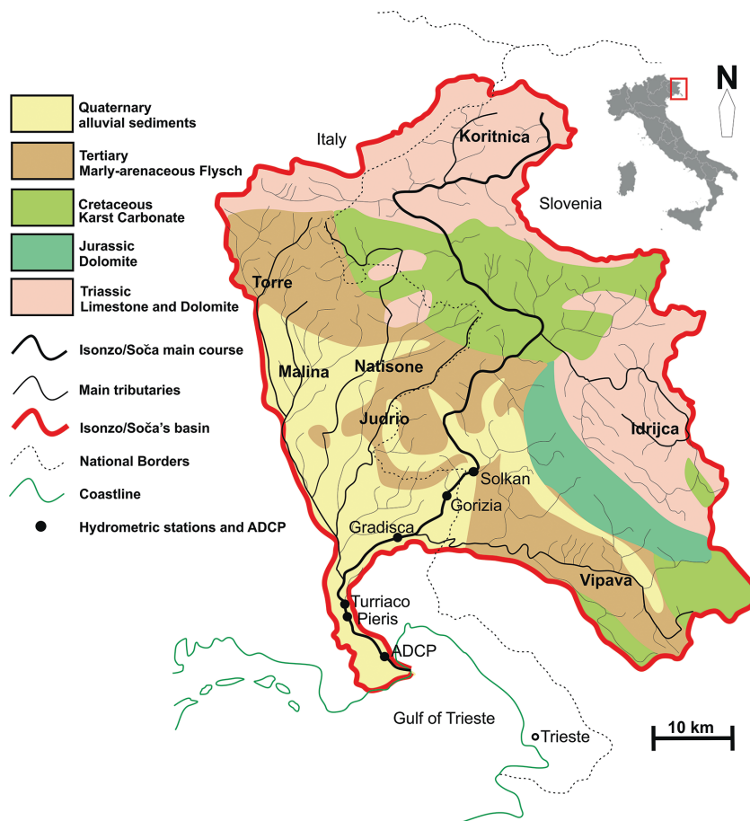
Fig. 1 - Schematic hydrogeological map of the Isonzo River basin, with the gauging and ADCP stations considered in the study [modified from Comici and Bussani (2007); schematic geological map of the Slovenian portion from Szeramek et al. (2011), schematic geological map of the Italian portion from Fontana et al. (2019)]. The hydrographic network was adapted from the EU-Hydro River Network Database 2006-2012 (vector), Europe – Shapefile (doi: 10.2909/393359a7-7ebd-4a52-80ac-1a18d5f3db9c), downloaded from https://land.copernicus.eu/en/map-viewer . The basin boundaries were adapted from those reported in Autorità di Bacino di Isonzo, Tagliamento, Livenza, Piave e Brenta-Bacchiglione e Autorità di Bacino dell'Adige (2014).
