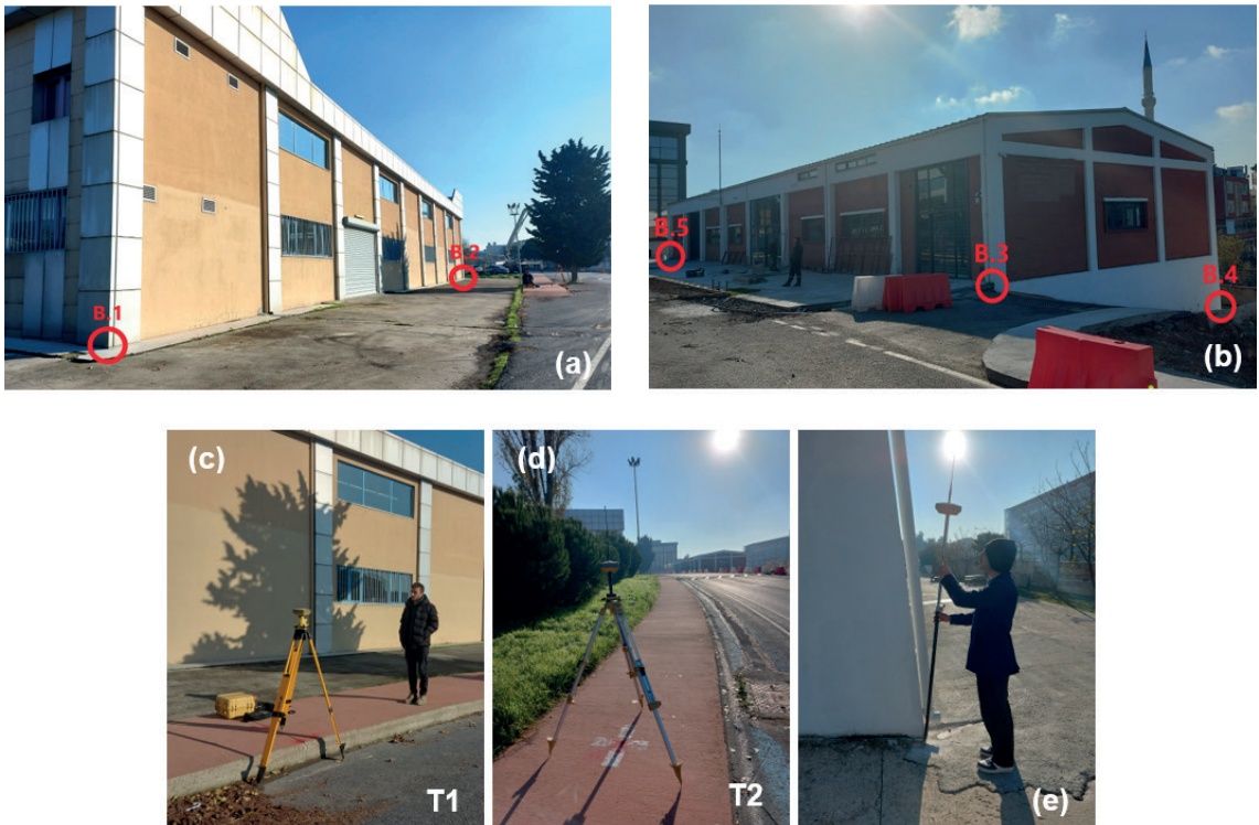
Fig. 5 - The B1, B2, B3, B4, and B5 corner points (panels a and b) and T1 and T2 reference points (panels c and d) in the study region and TILT surveying (panel e).
