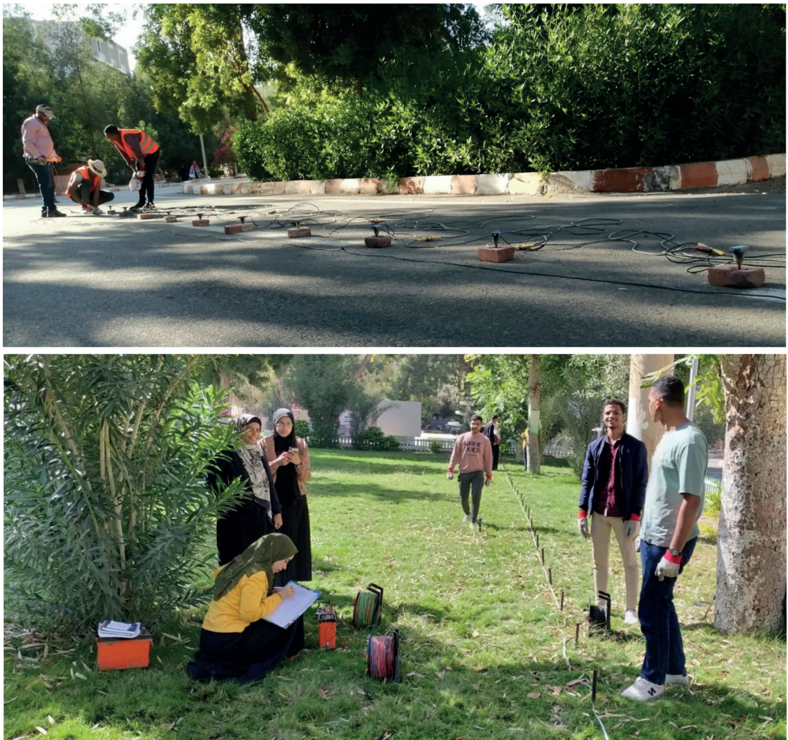
Fig. 4 - Images show the acquisition of the SRT and ERT data. The upper image shows the acquisition of the seismic data on the asphalt road, where the geophones are inserted on concrete blocks. The lower image shows ERT line acquisition within the garden. The geology and geophysics students of the faculty of sciences assisted in the acquisition process.
