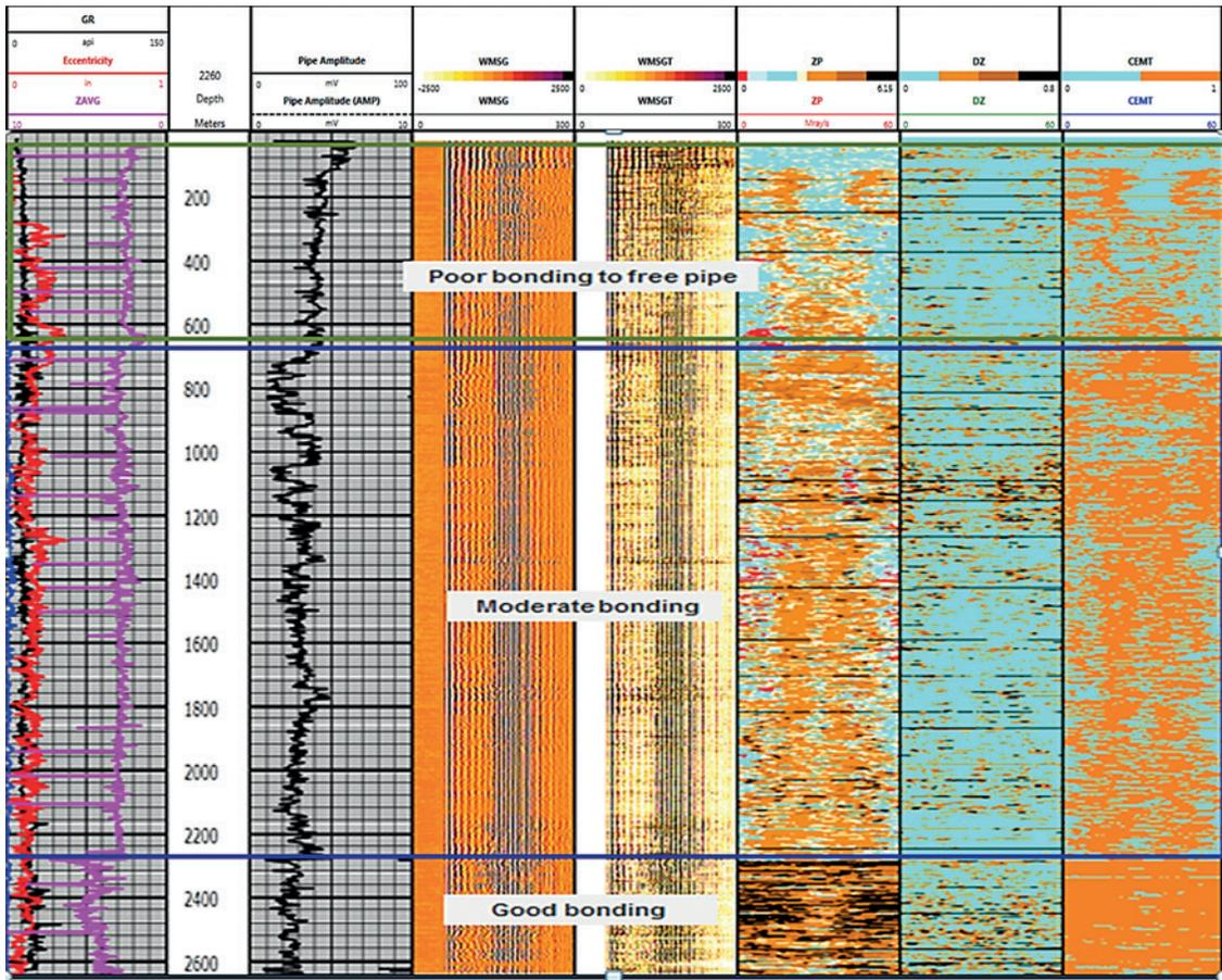
Fig. 12 - Cement evaluation by CBL-VDL CAST log for 9.625" open hole (WQ1-XX2).
