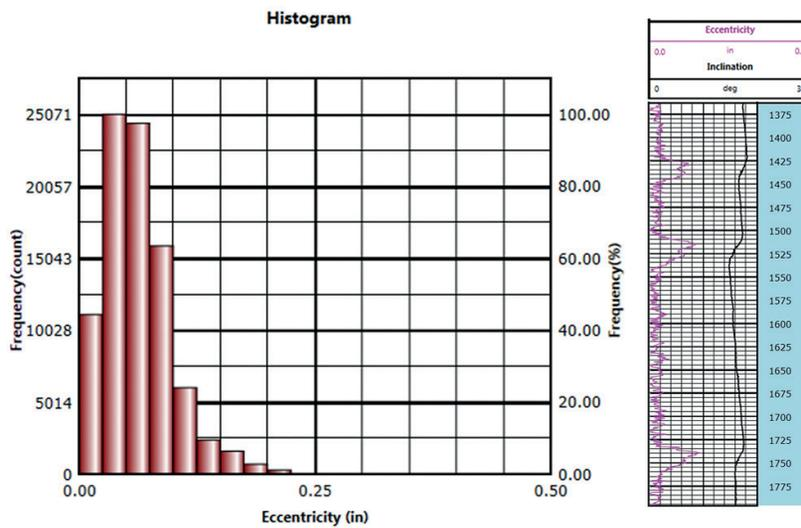
Fig. 15 - The eccentricity of the logging tool for well WQ1-XX0: left) the histogram showing the frequency and right) showing the log.
