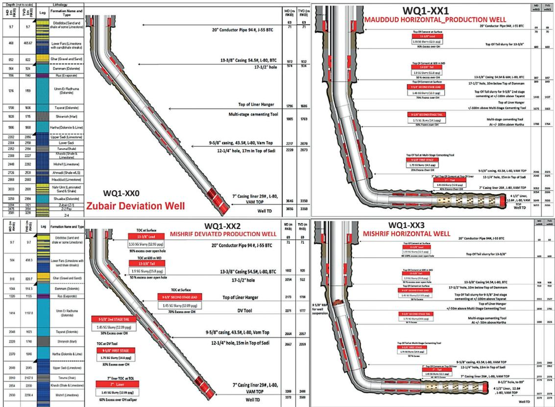
Fig. 5 - Well scheme and lithology by Powerdraw™.
