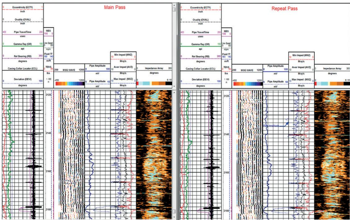
Fig. 16 - CBL-VDL CAST log for 7" open hole for well WQ1-XX0 (main and repeat pass).
