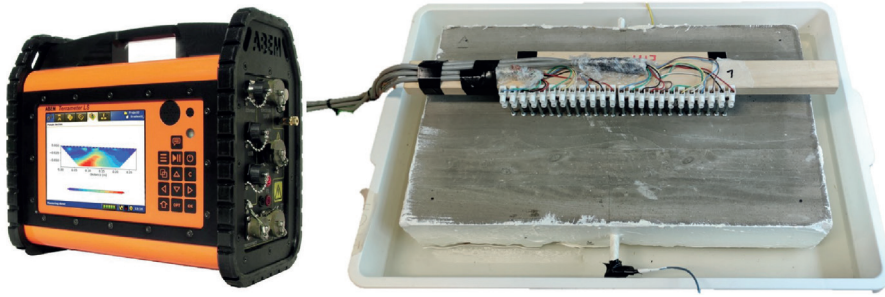
Fig. 4 - Multi-electrode resistivity probe developed for ERT measurements. The ERT survey was acquired using the ABEM Terrameter LS02 instrument connected to 24 steel nails, acting as electrodes.
